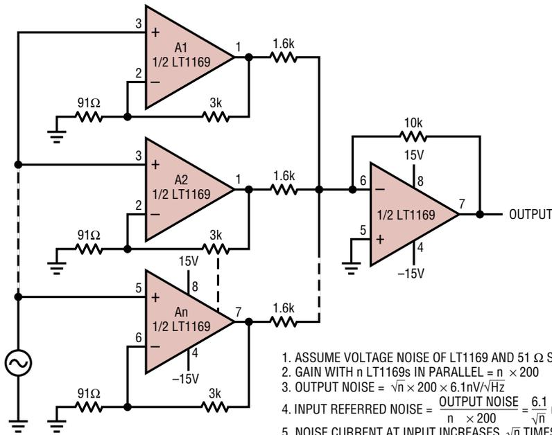
1. ASSUME VOLTAGE NOISE OF LT1169 AND  $51\Omega$  SOURCE RESISTOR =  $6.1nV/\sqrt{Hz}$
