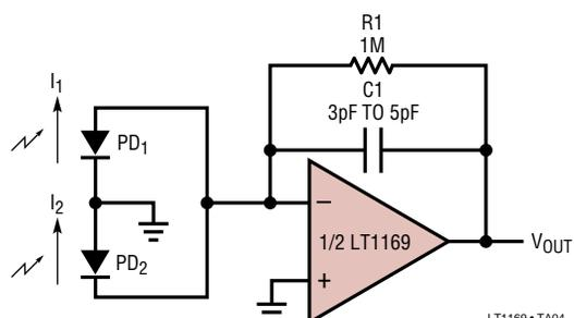
$V_{OUT} = 1M \times (I_1 - I_2)$
