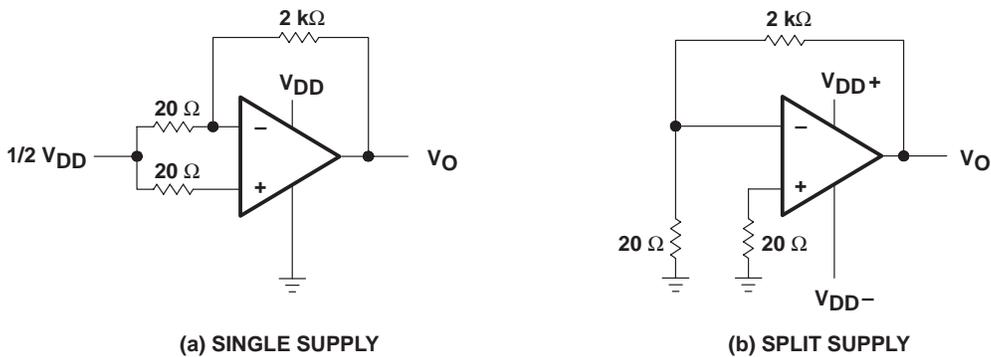
Figure 2. Noise-Test Circuit
