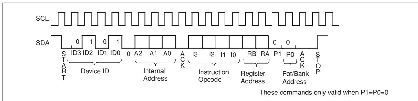
Figure 4. Three-Byte Instruction Sequence
