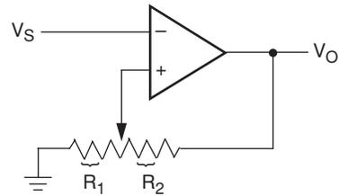
$$V_{UL} = \{R_1/(R_1 + R_2)\} V_O(\text{max})$$
