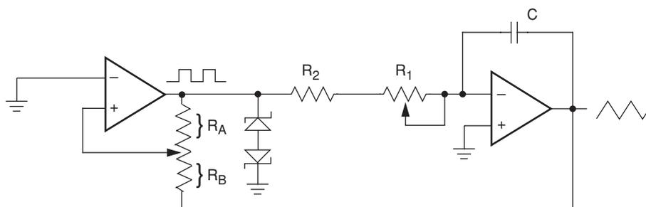
$$\text{frequency} \propto R_1, R_2, C$$
