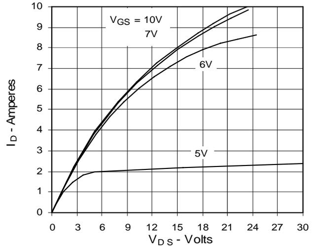
**Fig. 3. Output Characteristics**
