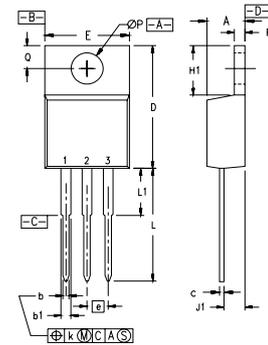
Pin 1 - Gate, Pin 2 - Source, Pin 3 - Drain, Pin 4 - Drain
