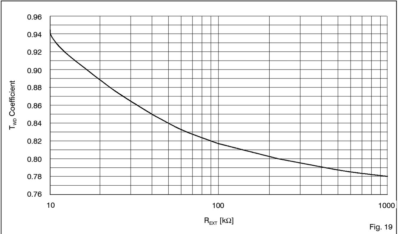
**$R_{EXT}$  Coefficient versus  $T_{WD}$  at  $T_J = + 25\text{ }^\circ\text{C}$**
