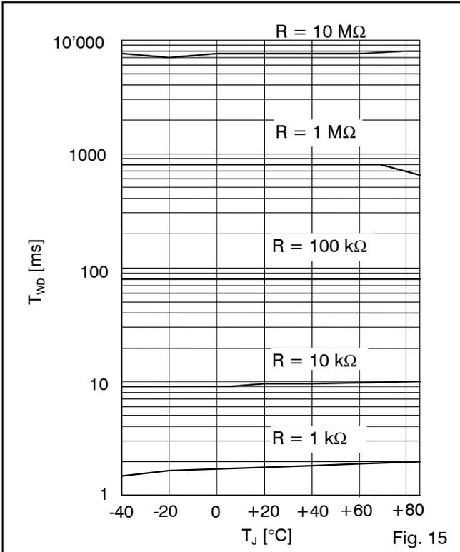
$T_{WD}$  versus R at 5 V
