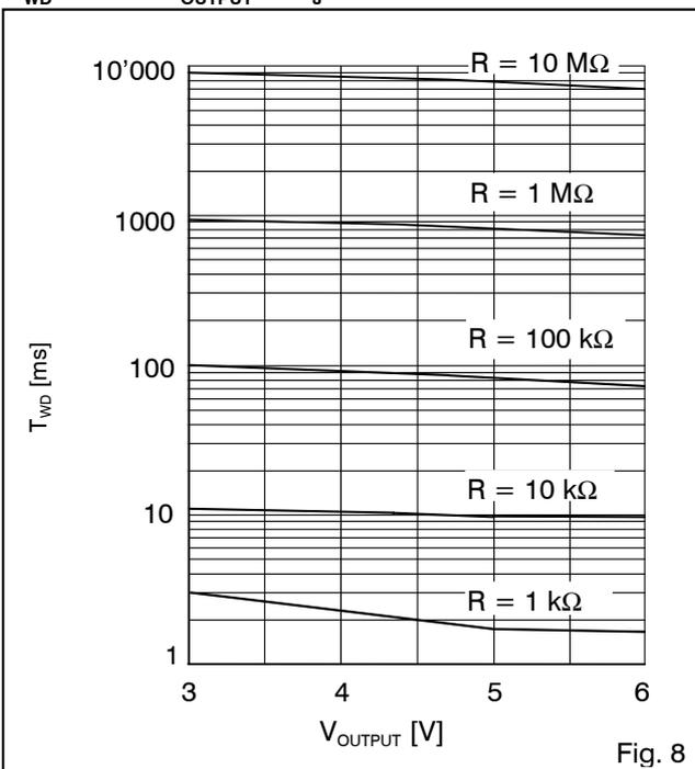
**$T_{WD}$  versus  $R$  at  $T_J = +25$  °C**
