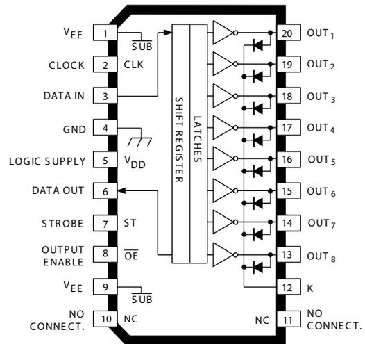
Note the 18-pin DIP package and the SOIC packages are electrically identical and share common terminal number assignments.
