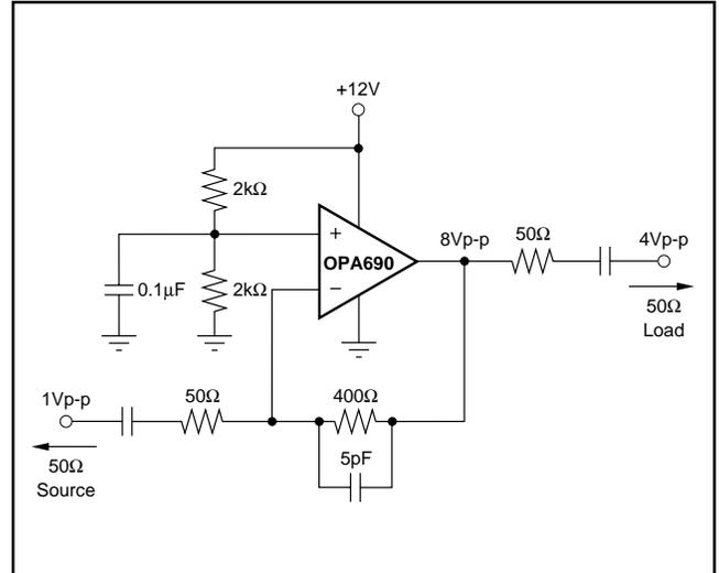
FIGURE 6. High Power Coax Line Driver.
