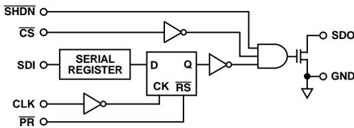
Figure 19. Detail SDO Output Schematic of the AD5204
