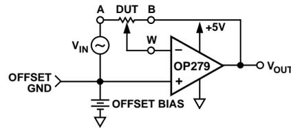
Figure 26. Inverting Programmable Gain Test Circuit
