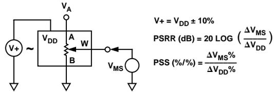
Figure 25. Power Supply Sensitivity Test Circuit (PSS, PSRR)
