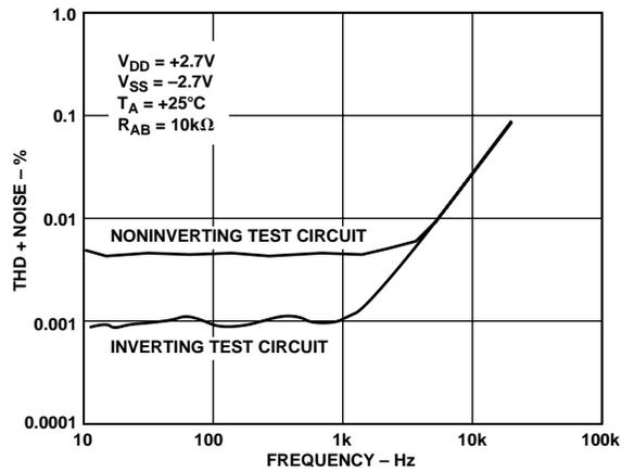
Figure 15. Total Harmonic Distortion Plus Noise vs. Frequency
