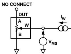
Figure 23. Resistor Position Nonlinearity Error (Rheostat Operation; R-INL, R-DNL)
