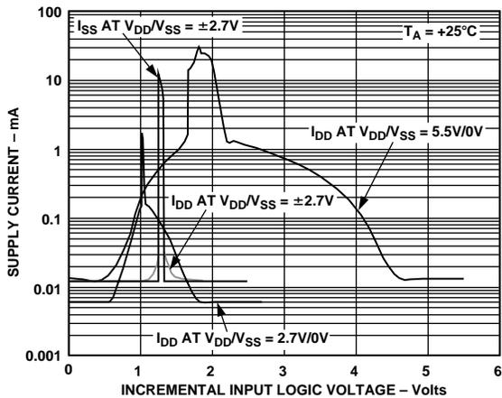
Figure 12. Supply Current vs. Input Logic Voltage
