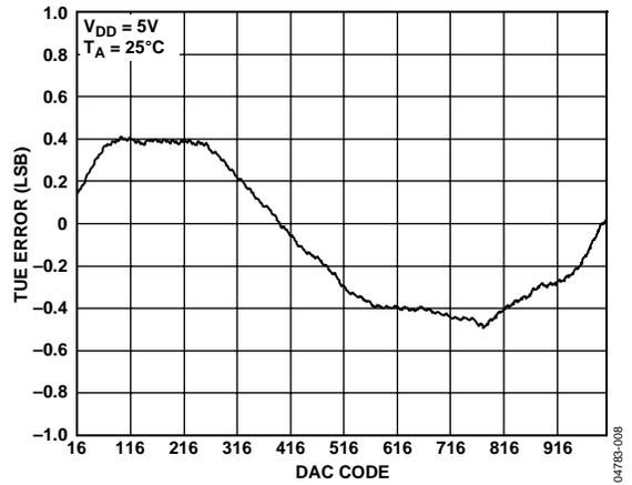
Figure 8. AD5611 Total Unadjusted Error (TUE)
