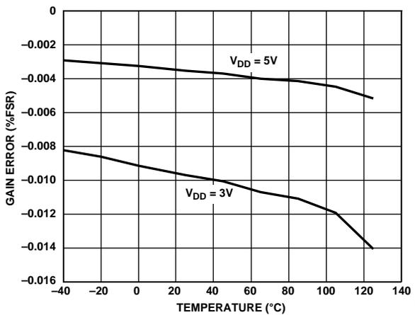
Figure 30. Gain Error vs. Temperature (5 V)
