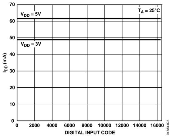
Figure 23. Supply Current vs. Digital Input Code
