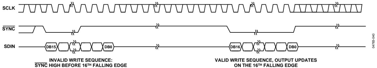
Figure 43.  $\overline{SYNC}$  Interrupt Facility
