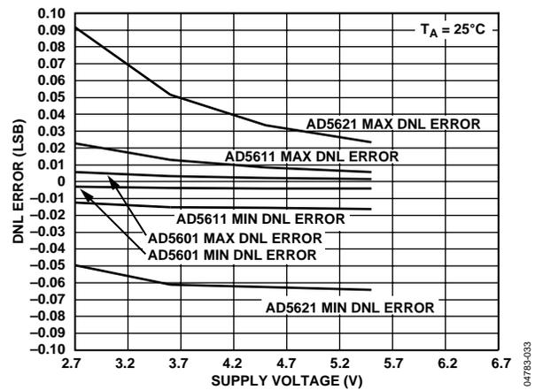
Figure 33. DNL vs. Supply Voltage at 25°C
