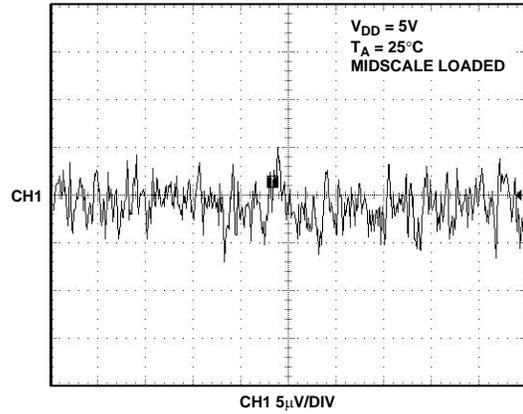
Figure 19. 1/f Noise, 0.1 Hz to 10 Hz Bandwidth
