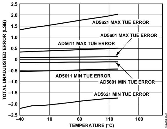
Figure 28. Total Unadjusted Error (TUE) vs. Temperature (5 V)
