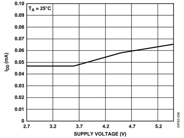
Figure 36. Supply Current vs. Supply Voltage at 25°C
