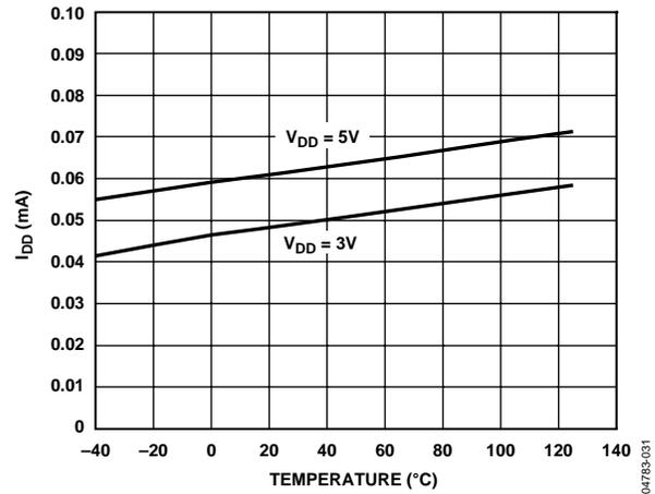
Figure 31. Supply Current vs. Temperature (5 V)
