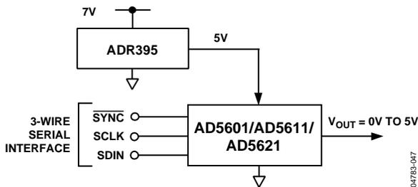
Figure 50. ADR395 as Power Supply to the AD5601/AD5611/AD5621
