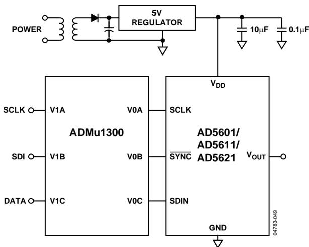
Figure 52. AD5601/AD5611/AD5621 with a Galvanically Isolated Interface
