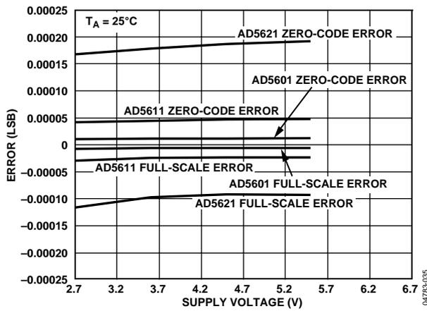
Figure 35. Zero-Code and Full-Scale Error vs. Supply Voltage at 25°C
