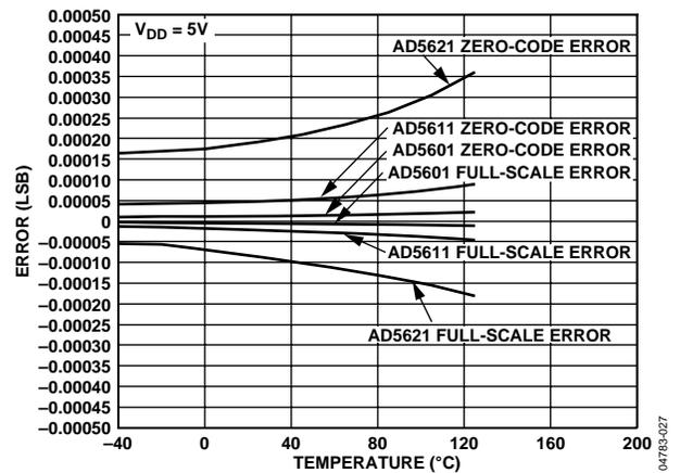
Figure 27. Zero-Code and Full-Scale Error vs. Temperature
