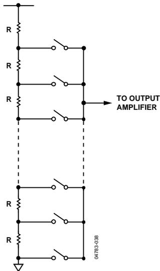
Figure 39. Resistor String Structure
