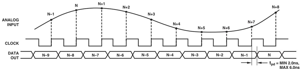
Figure 1. Timing Diagram
