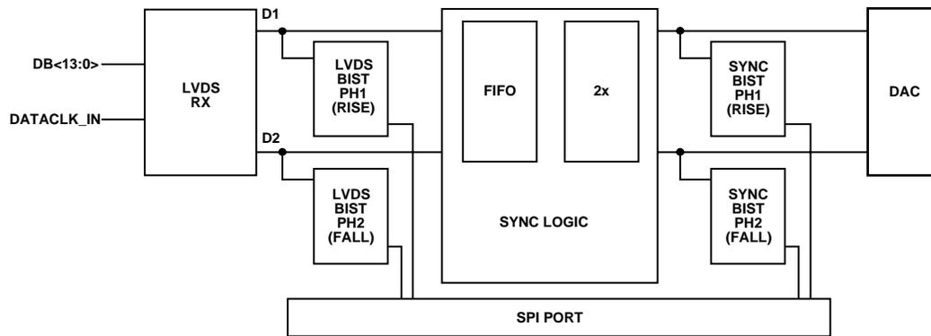
Figure 82. Block Diagram Showing LVDS and Sync Phase 1 and Phase 2
