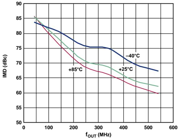
Figure 44. AD9736 IMD vs.  $f_{OUT}$  over Temperature, 1.2 GSPS
