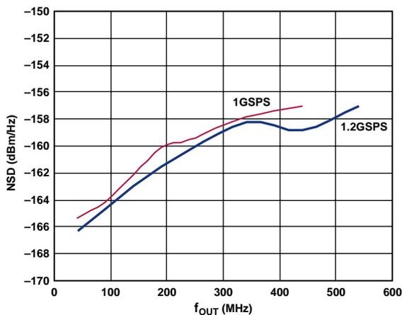
Figure 51. AD9736 1-Tone NSD vs.  $f_{OUT}$  over  $f_{DAC}$ , 25°C
