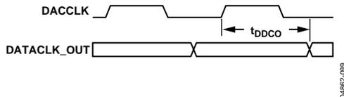
Figure 99. DACCLK to DATACLK\_OUT Delay
