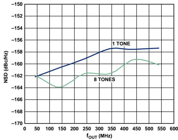
Figure 64. AD9735 NSD vs.  $f_{OUT}$ , 1.2 GSPS
