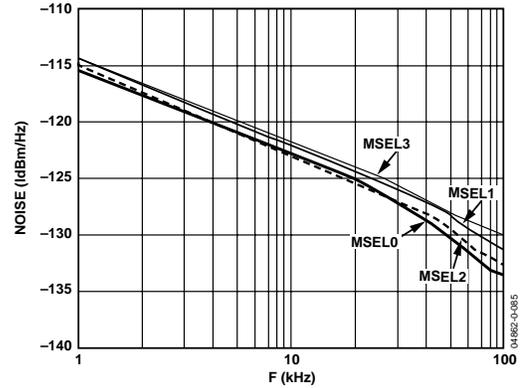
Figure 85. 1/f Noise with Respect to MSEL Bits
