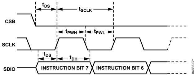
Figure 71. Timing Diagram for SPI Register Write
