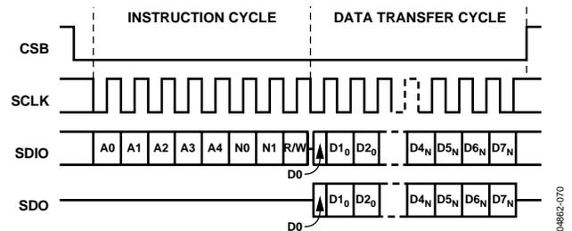
Figure 70. Serial Register Interface Timing, LSB-First Read
