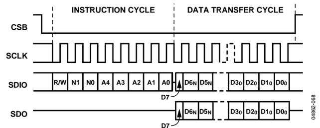
Figure 68. Serial Register Interface Timing, MSB-First Read
