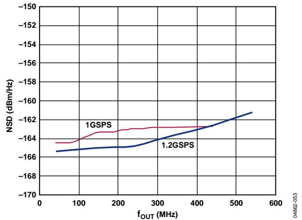
Figure 53. AD9736 8-Tone NSD vs.  $f_{OUT}$  over  $f_{DAC}$ , 25°C
