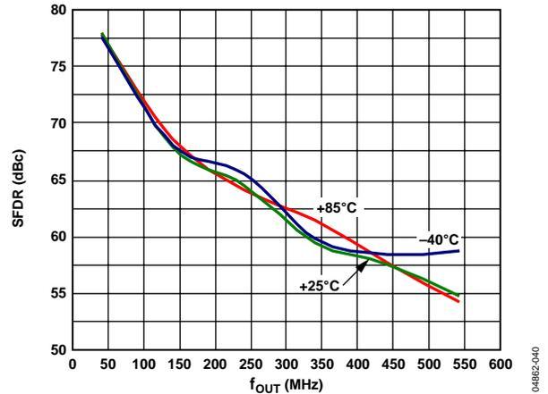
Figure 40. AD9736 SFDR vs.  $f_{OUT}$  over Temperature
