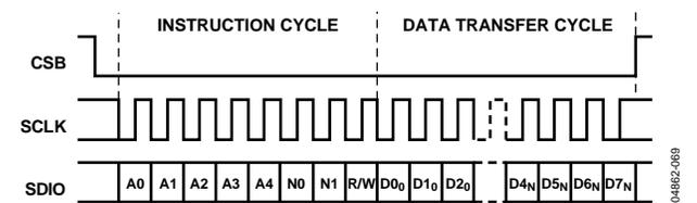
Figure 69. Serial Register Interface Timing, LSB-First Write
