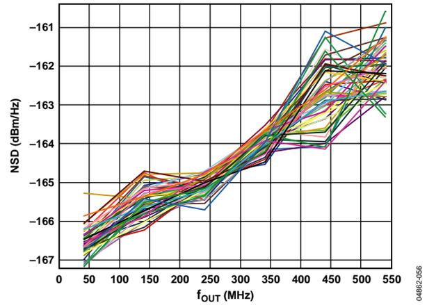
Figure 56. AD9736 1-Tone NSD vs.  $f_{OUT}$  over 50 Parts, 1.2 GSPS, 25°C
