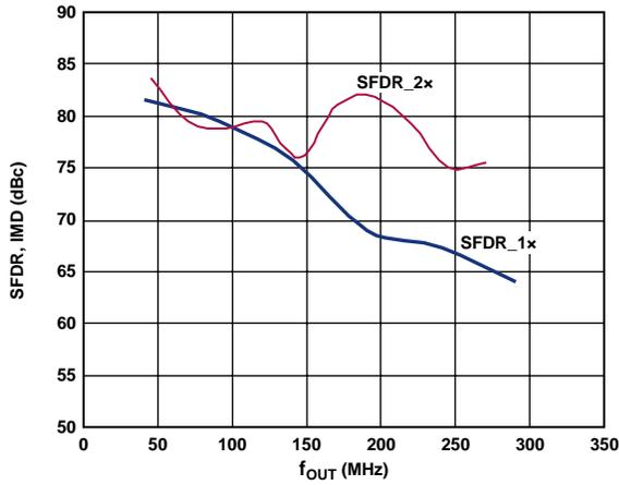
Figure 49. AD9736 SFDR vs.  $f_{OUT}$ , 25°C, 1.2 GSPS, 1x and 2x Interpolation
