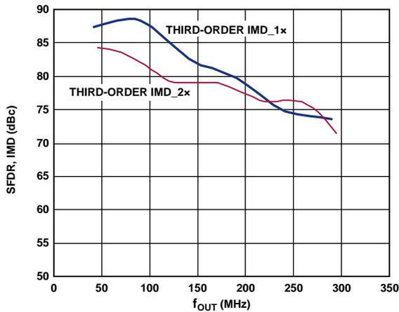
Figure 50. AD9736 IMD vs.  $f_{OUT}$ , 25°C, 1.2 GSPS, 1x and 2x Interpolation
