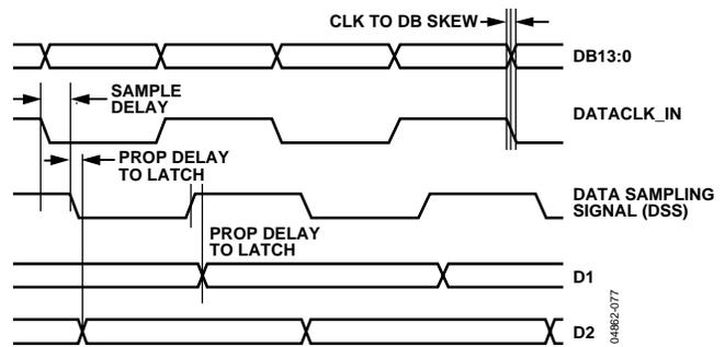
Figure 77. AD973x Internal LVDS Data Sampling Logic Timing
