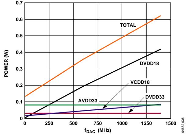
Figure 38. AD9736 2x Interpolation Mode Power vs.  $f_{DAC}$  at 25°C
