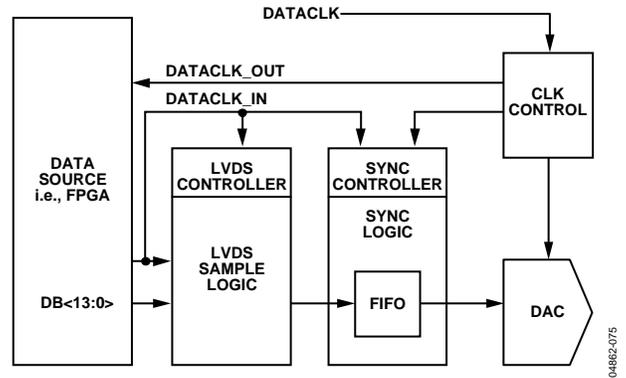
Figure 75. AD973x Data Controllers
