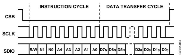
Figure 67. Serial Register Interface Timing, MSB-First Write
