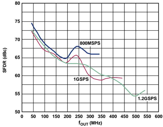
Figure 60. AD9735 SFDR vs.  $f_{OUT}$  over  $f_{DAC}$ , 1.2 GSPS
