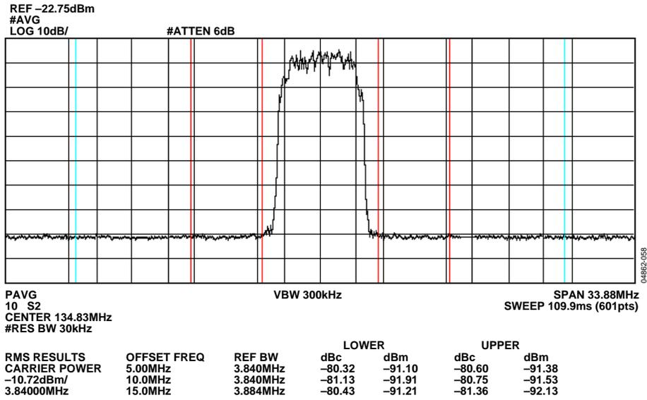
Figure 58. AD9735 WCDMA Carrier at 134.83 MHz,  $f_{DAC} = 491.52$  MSPS
