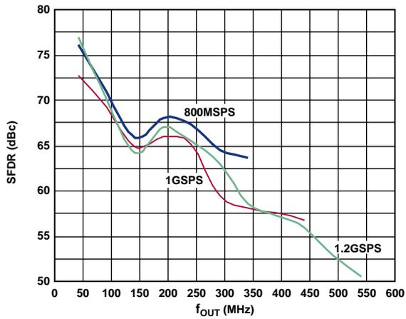
Figure 61. AD9734 SFDR vs.  $f_{OUT}$  over  $f_{DAC}$ , 1.2 GSPS
