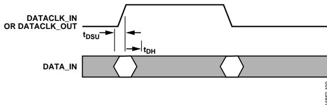
Figure 100. Standard Definitions for DATACLK\_IN or DATACLK\_OUT to Data Setup and Hold,  $SD = 0$
