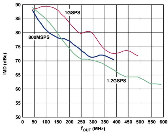
Figure 62. AD9735 IMD vs.  $f_{OUT}$  over  $f_{DAC}$ , 1.2 GSPS
