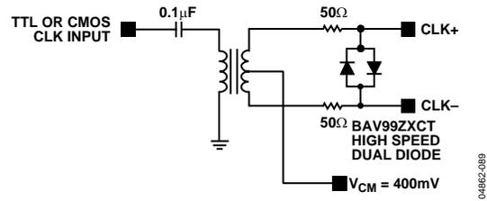
Figure 89. TTL or CMOS DACCLK Drive Circuit
