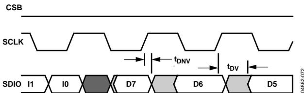
Figure 72. Timing Diagram for SPI Register Read
