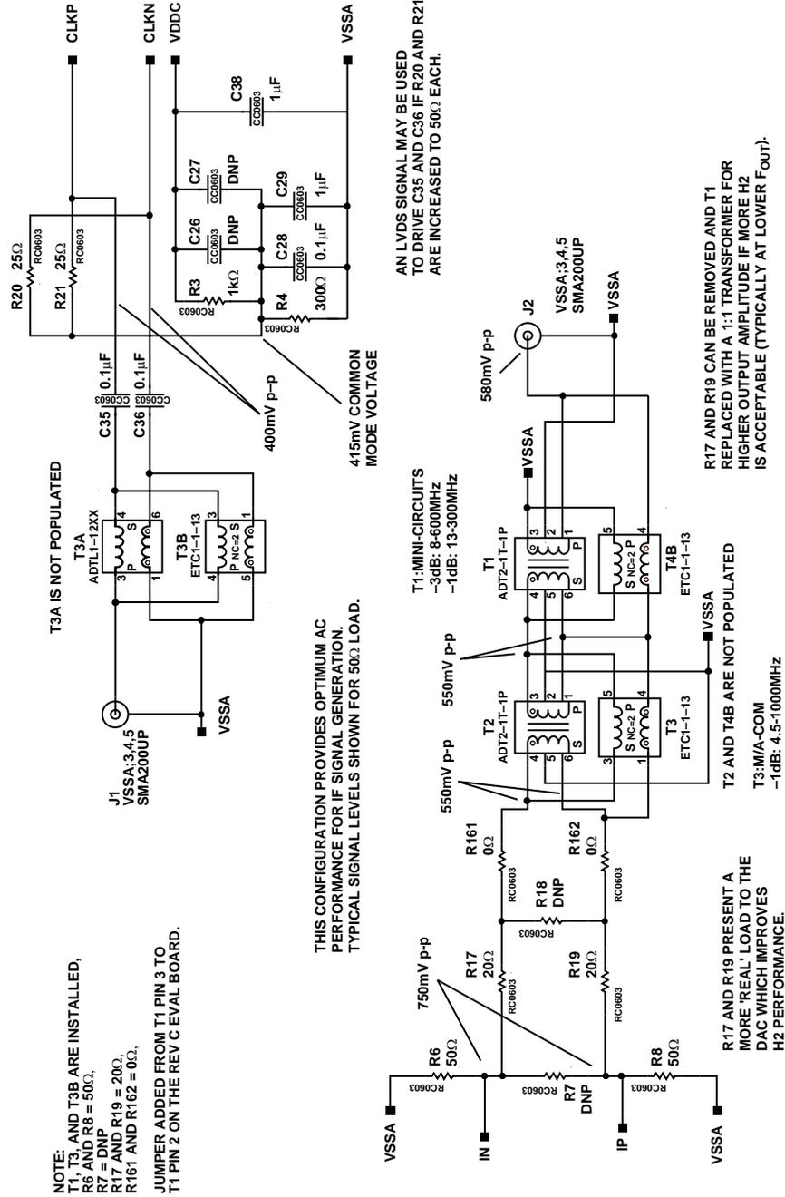
Figure 105. Clock Input and Analog Output, AD973x Evaluation Board, Rev. F
