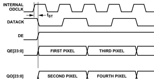
Figure 40. Two Pixels per Clock (DATAACK Inverted)
