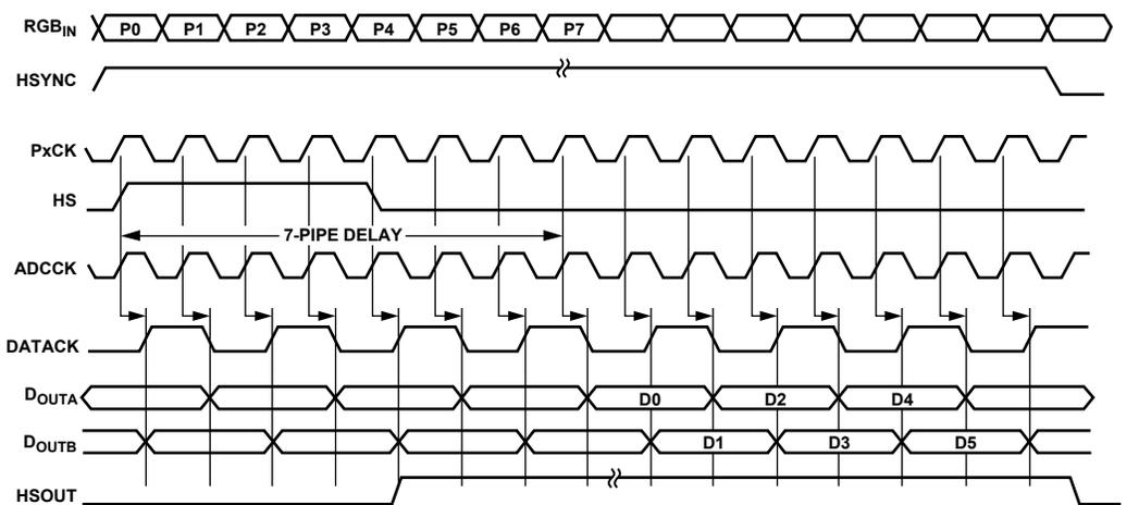
Figure 21. Dual-Channel Mode, Interleaved Outputs (Analog Interface), Outphase = 0
