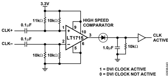
Figure 28. External Digital Interface Clock Detect Circuit
