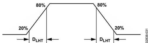
Figure 33. Digital Output Rise and Fall Times
