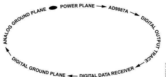
Figure 44. Example of a Current Loop
