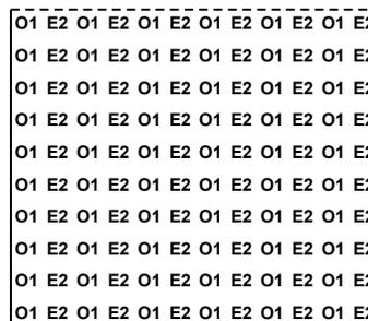
Figure 15. Combine Frame Output from Graphics Controller
