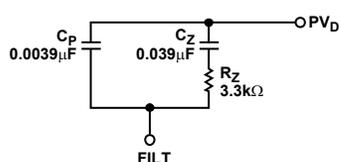
Figure 11. PLL Loop-Filter Detail
