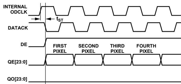
Figure 38. One Pixel per Clock (DATAACK not Inverted)
