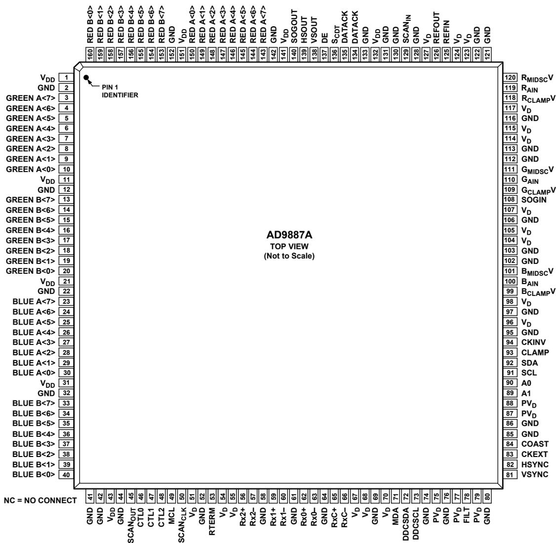
Figure 2. Pin Configuration
