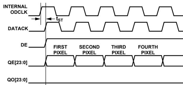
Figure 37. One Pixel per Clock (DATAACK Inverted)
