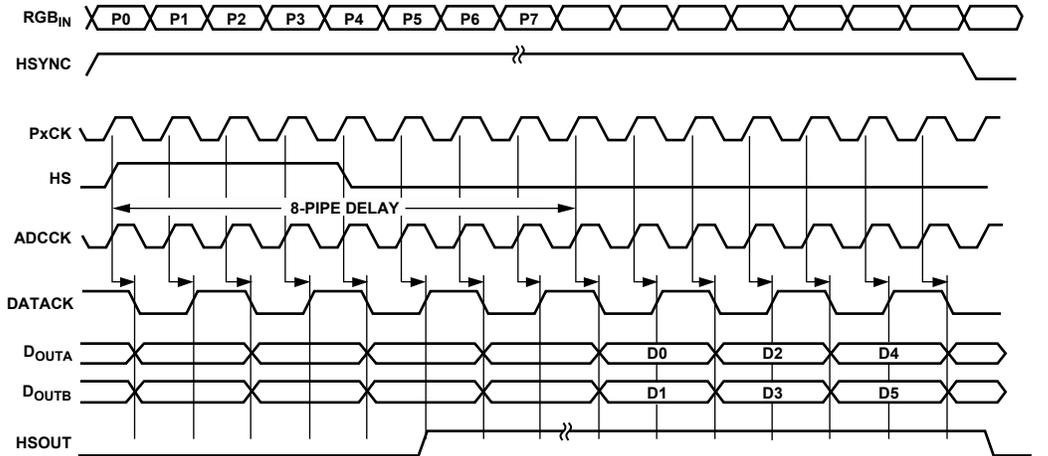
Figure 22. Dual-Channel Mode, Parallel Outputs (Analog Interface), Outphase = 0
