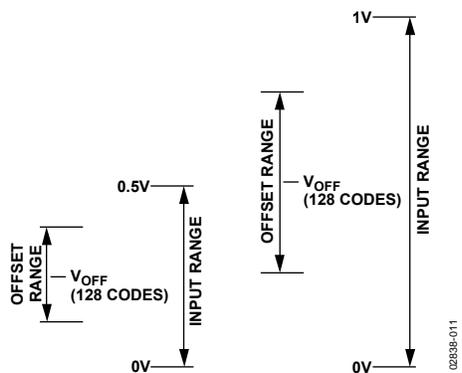
Figure 7. Relationship of Offset Range to Input Range
