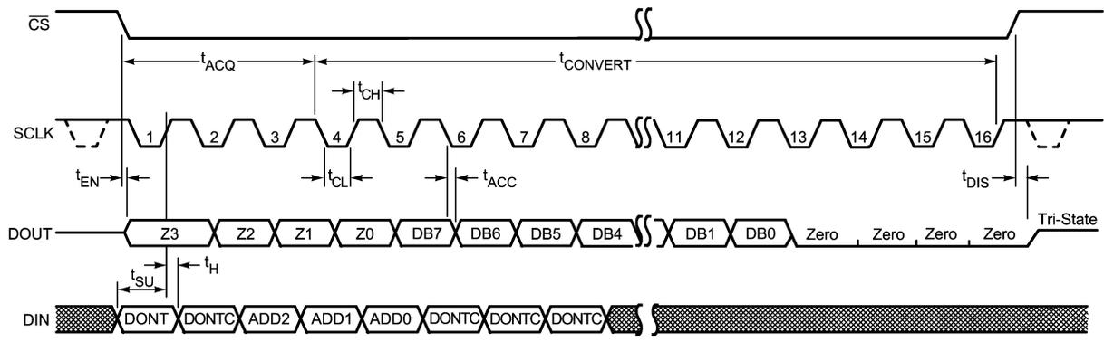
ADC082S021 Serial Timing Diagram
