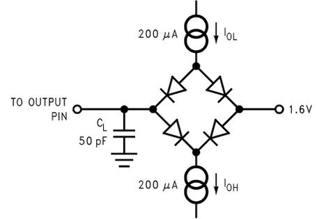
Timing Test Circuit
