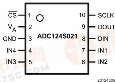
ADC124S021 4 Channel, 200 kSPS, 12-Bit A/D Converter
