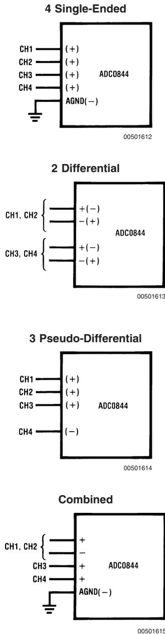
FIGURE 1. Analog Input Multiplexer Options
