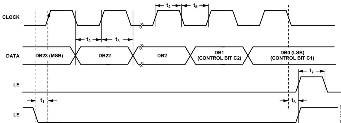
Figure 2. Timing Diagram
