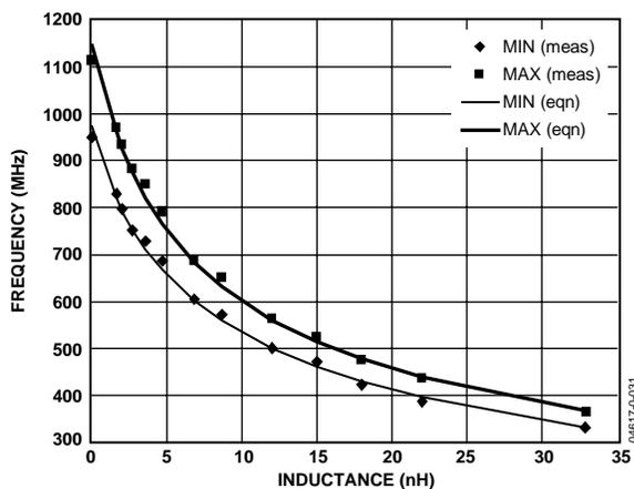
Figure 36. Output Frequency vs. External Inductor Value
