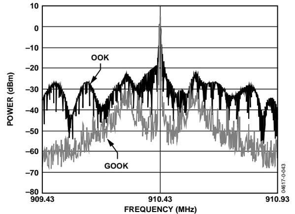
Figure 33. GOOK vs. OOK Frequency Spectra (Narrow-Band Measurement)
