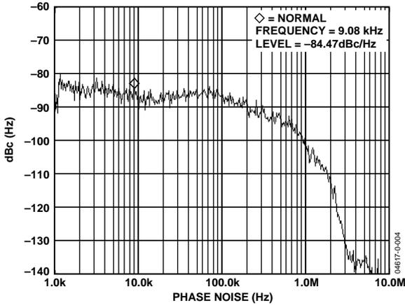
Figure 4. Phase Noise Response— $DV_{DD} = 3.0\text{ V}$ ,  $I_{CP} = 0.86\text{ mA}$ ,  $I_{VCO} = 2.0\text{ mA}$ ,  $F_{OUT} = 315\text{ MHz}$ ,  $PF_D = 3.6864\text{ MHz}$ ,  $PA\text{ Bias} = 5.5\text{ mA}$
