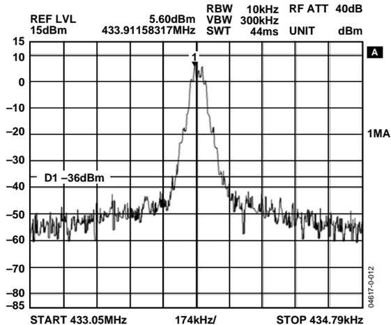
Figure 12. FSK Modulation, Power = 10 dBm, Data Rate = 38.4 kbps,  $F_{DEVIATION} = \pm 19.28 \text{ kHz}$
