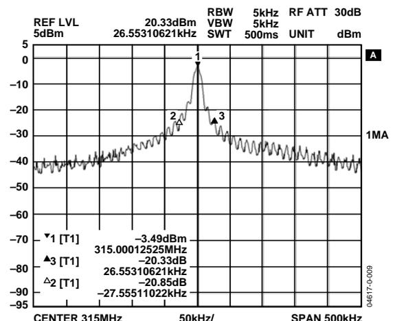
Figure 9. OOK Modulation, Power = 0 dBm, Data Rate = 10 kbps
