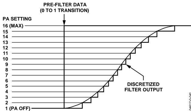
Figure 32. Varying PA Output for GOOK (Index Counter = 16).
