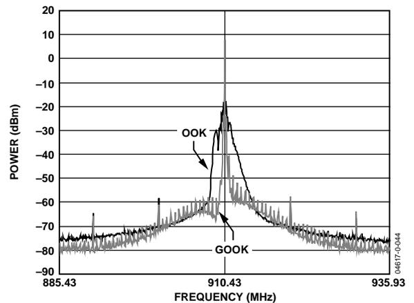
Figure 34. GOOK vs. OOK Frequency Spectra (Wideband Measurement)
