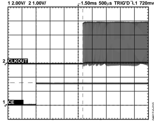
Figure 10. Crystal Power-On Time, 4 MHz, Time = 1.6 ms
