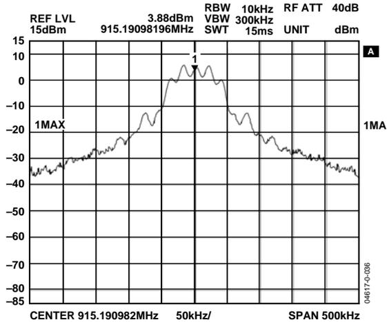
Figure 22. FSK Modulation,  $P_{ower} = 10 \text{ dBm}$ ,  $D_{ata \text{ Rate}} = 38.4 \text{ kbps}$ ,  $F_{deviation} = \pm 19.2 \text{ kHz}$
