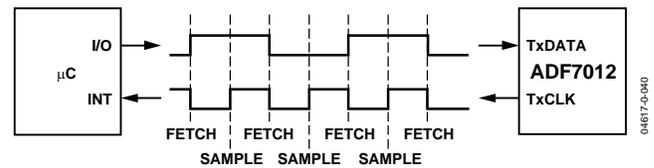
Figure 31. TxCLK/TxDATA Synchronization.
