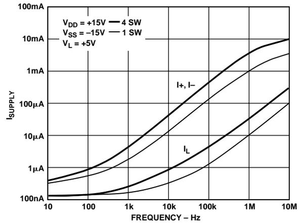
Figure 5. Supply Current vs. Input Switching Frequency
