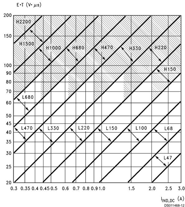
**Note:** These charts assume that the inductor ripple current is approximately 20% to 30% of the average inductor current (when the regulator is under full load). Greater ripple current causes higher peak switch currents and greater output ripple voltage; lower ripple current is achieved with larger-value inductors. The factor of 20 to 30% is chosen as a convenient balance between the two extremes.
