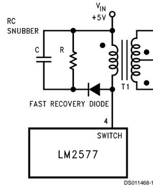
FIGURE 21. Snubber Circuit
