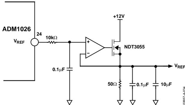
Figure 33.  $V_{REF}$  Interface Circuit for  $V_{REF}$  Loads  $> 2$  mA
