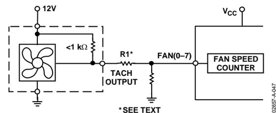
Figure 47. Fan with Strong Tach Pull-Up to > V<sub>CC</sub> or Totem Pole Output, Attenuated with R1/R2
