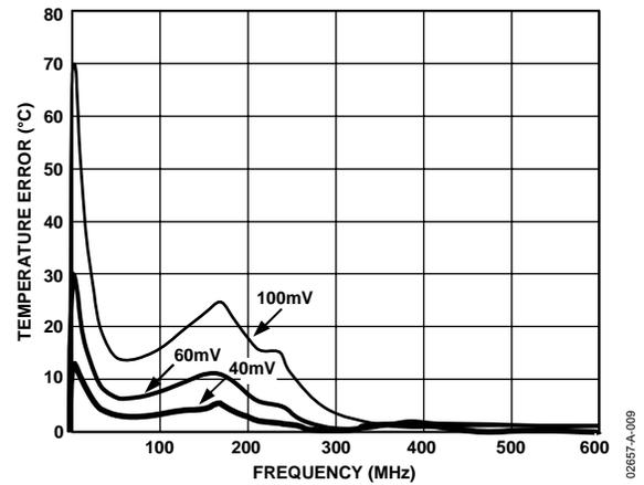
Figure 9. Temperature Error vs. Differential-Mode Noise Frequency
