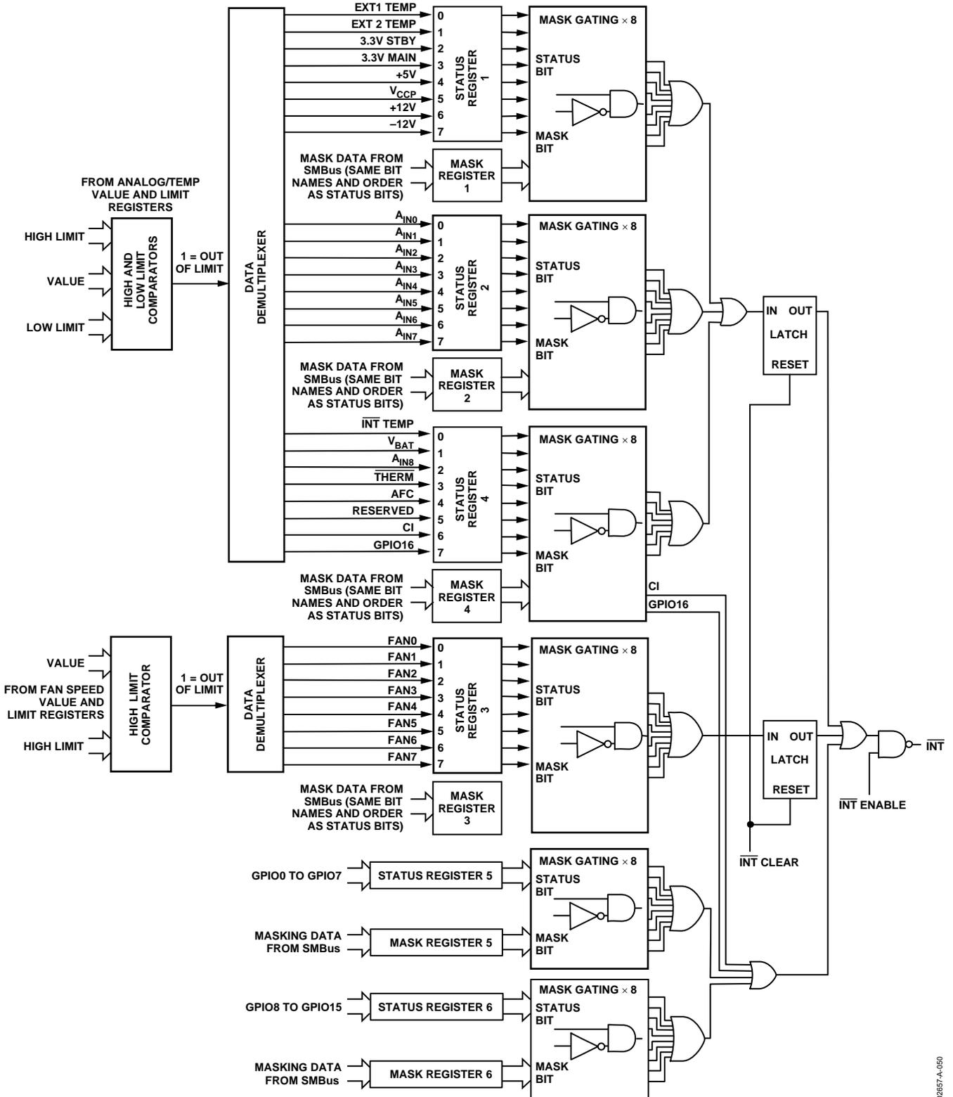
Figure 53. Interrupt Structure
