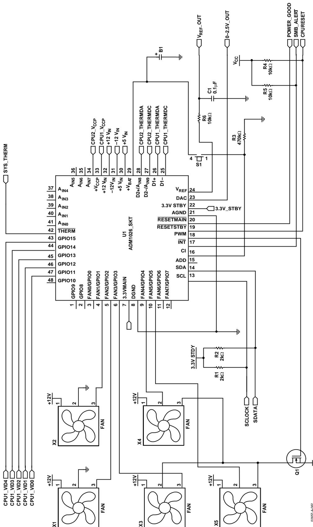
Figure 62. ADM1026 Schematic
