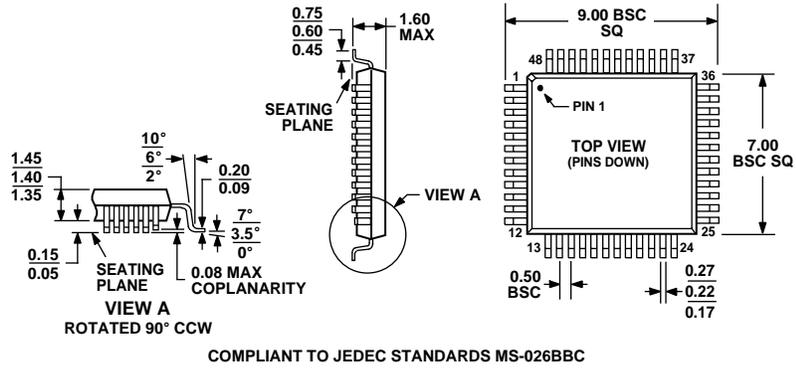
Figure 63. 48-Lead Thin Plastic Quad Flat Package [LQFP]
