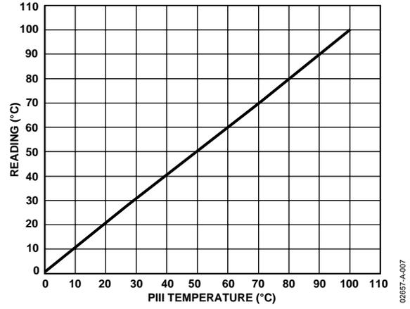
Figure 7. Pentium® III Temperature vs. ADM1026 Reading
