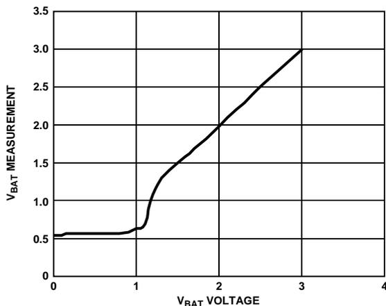
Figure 15. V<sub>BAT</sub> Measurement vs. Voltage
