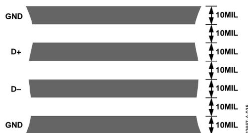
Figure 35. Arrangement of Signal Tracks
