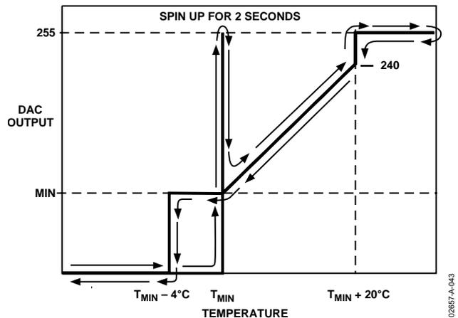
Figure 43. Automatic DAC Fan Control Transfer Function
