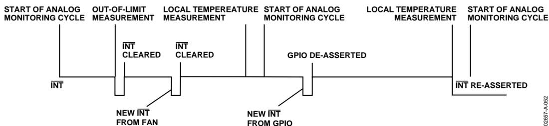
Figure 51. Other Interrupt Sources Can Reassert  $\overline{\text{INT}}$  Immediately
