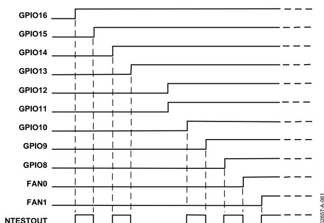
Figure 61. NAND Tree Test with Two Inputs Shorted
