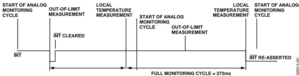
Figure 50. Delay After Clearing  $\overline{\text{INT}}$  Before Reassertion
