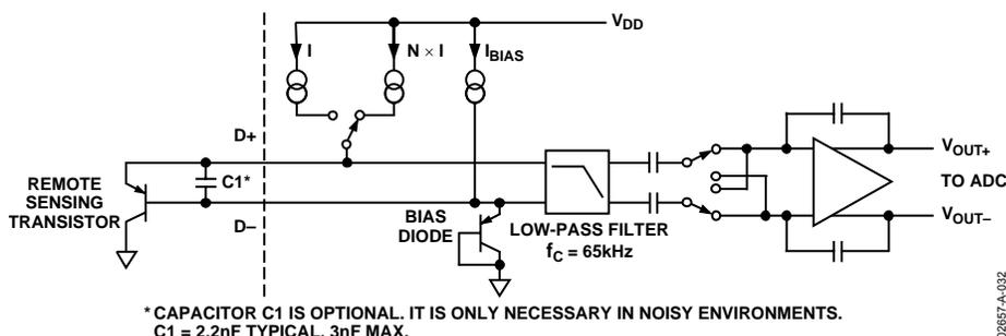
Figure 34. Signal Conditioning for Remote Diode Temperature Sensors
