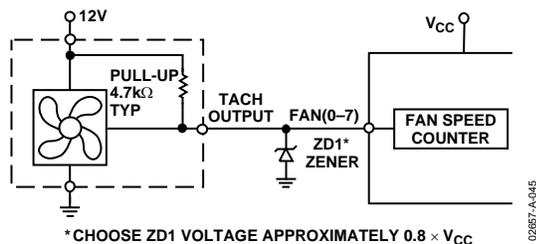
Figure 45. Fan with Tach Pull-Up to Voltage > V<sub>CC</sub> (e.g. 12 V), Clamped with Zener Diode
