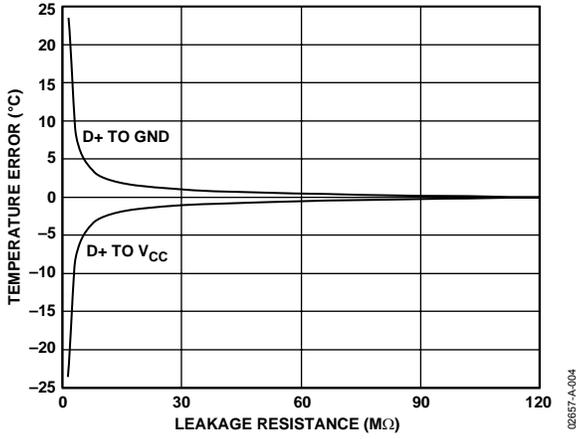
Figure 4. Temperature Error vs. PCB Track Resistance
