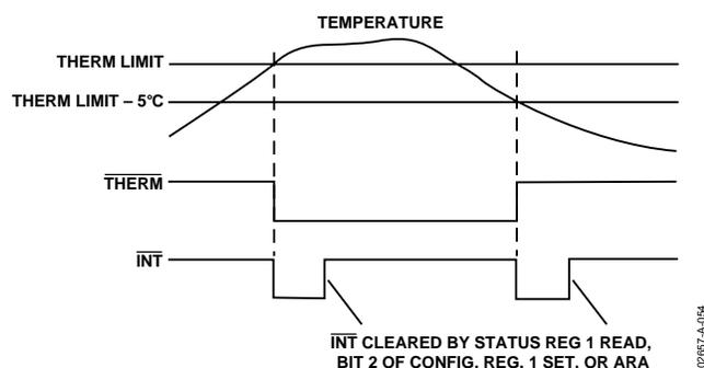
Figure 54. Assertion of  $\overline{\text{INT}}$  Due to  $\overline{\text{THERM}}$  Event
