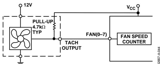
Figure 44. Fan with Tach Pull-Up to +V<sub>CC</sub>
