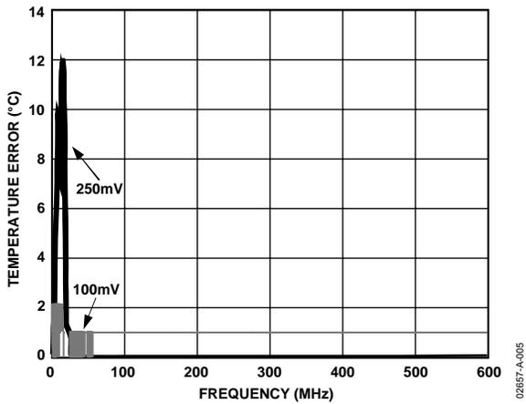
Figure 5. Temperature Error vs. Power Supply Noise Frequency
