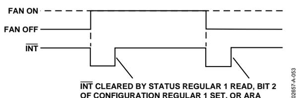
Figure 52. Assertion of  $\overline{\text{INT}}$  Due to AFC Event
