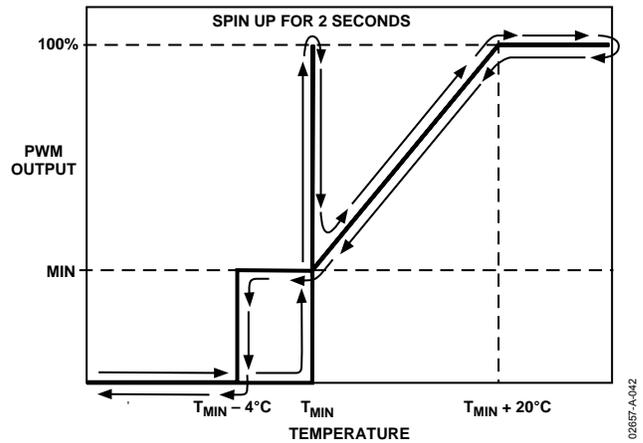
Figure 42. Automatic PWM Fan Control Transfer Function
