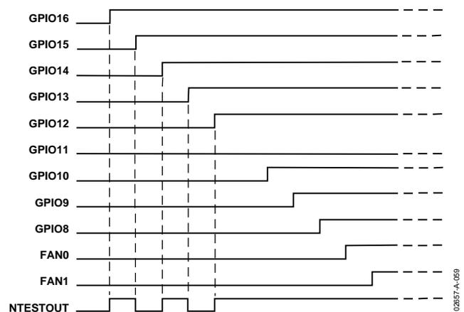
Figure 59. NAND Tree Test with GPIO11 Stuck Low
