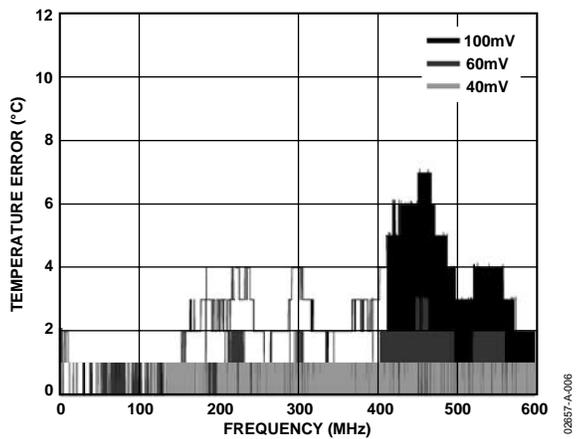
Figure 6. Temperature Error vs. Common-Mode Noise Frequency
