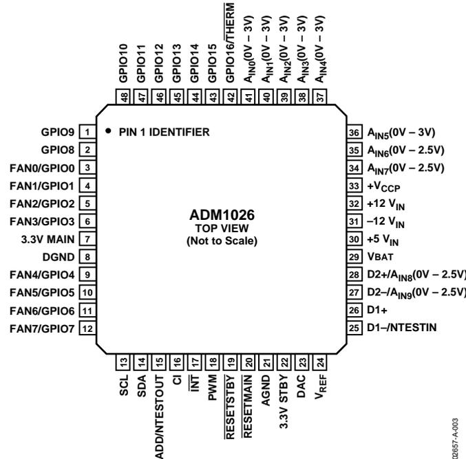
Figure 3. Pin Configuration
