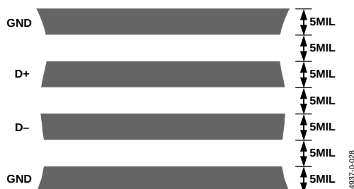
Figure 29. Arrangement of Signal Tracks
