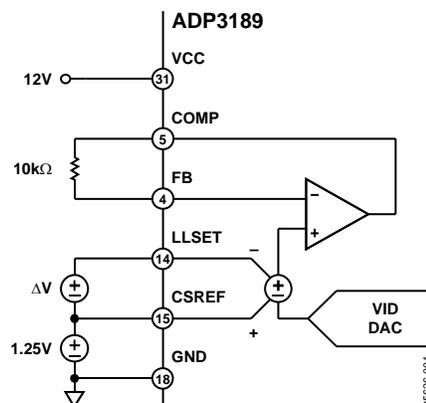
Figure 4. Positioning Voltage
