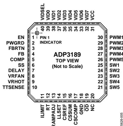
Figure 5. Pin Configuration
