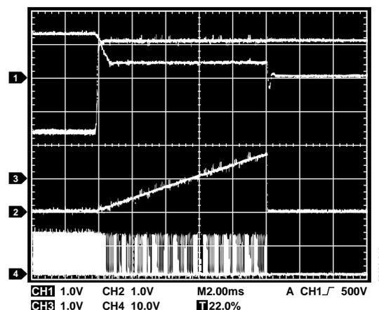
Figure 10. Overcurrent Latch-Off Waveforms
