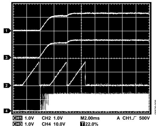
Figure 9. Typical Start-up Waveforms
