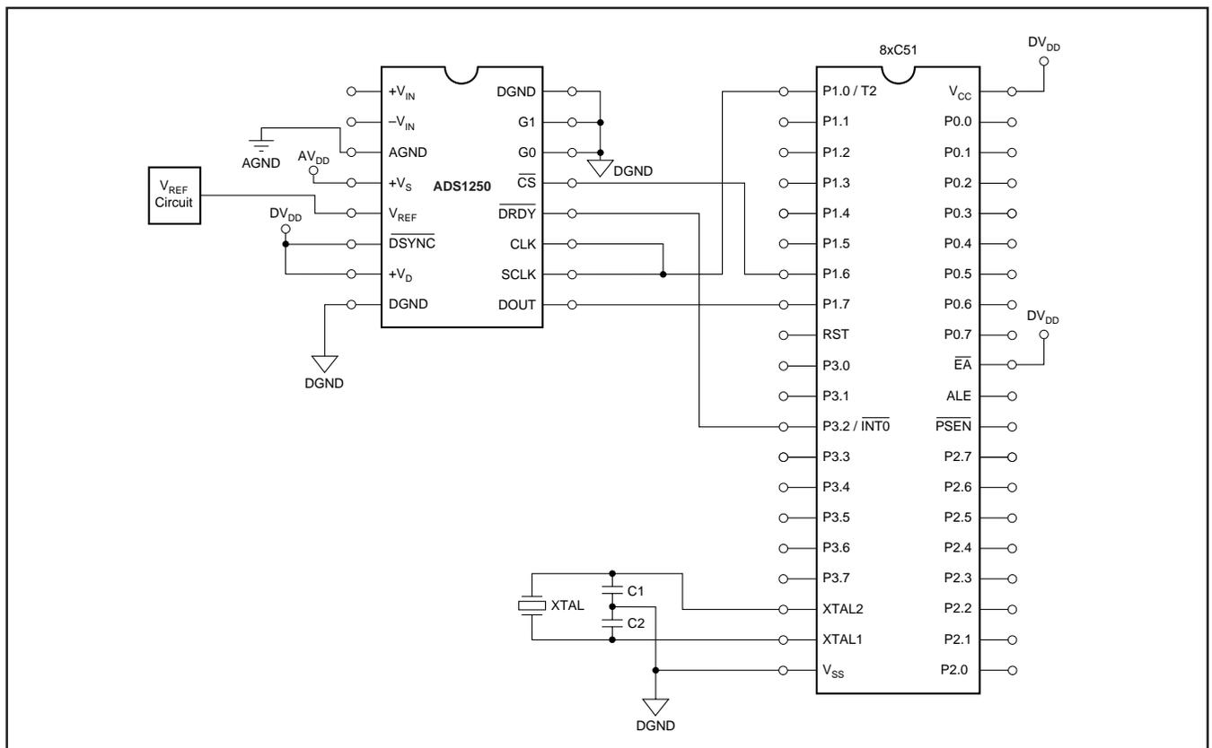
FIGURE 19. Four Wire Interface to an 8xC51 (Free Running SCLK)
