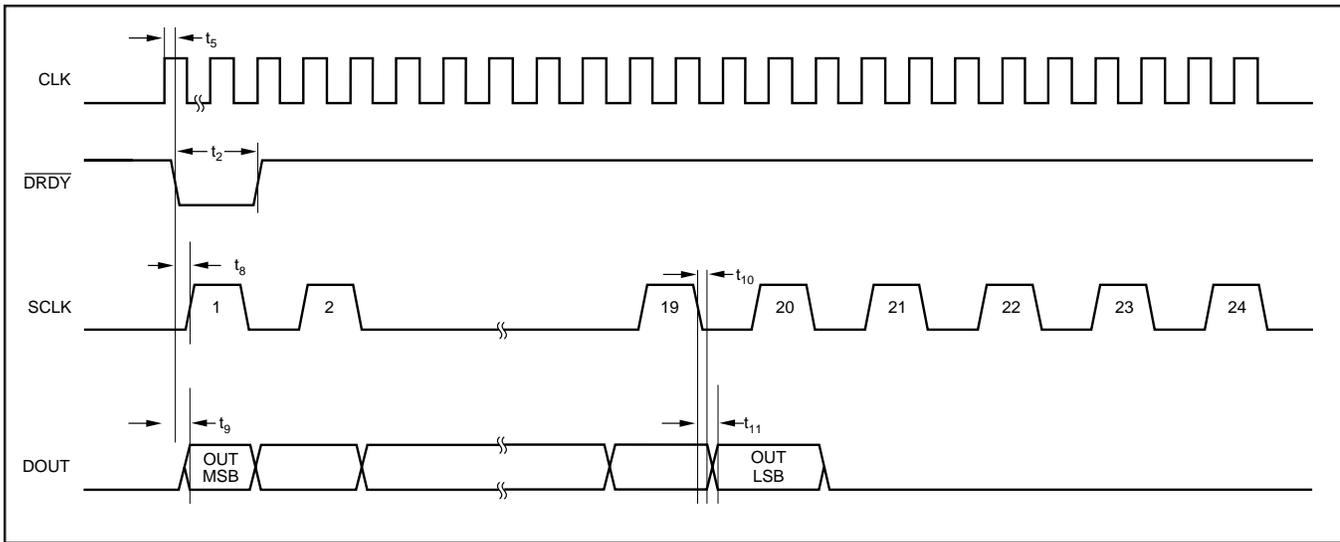
FIGURE 20. Method 3: Two-Wire Interface ( $\overline{\text{CS}}$  tied LOW).
