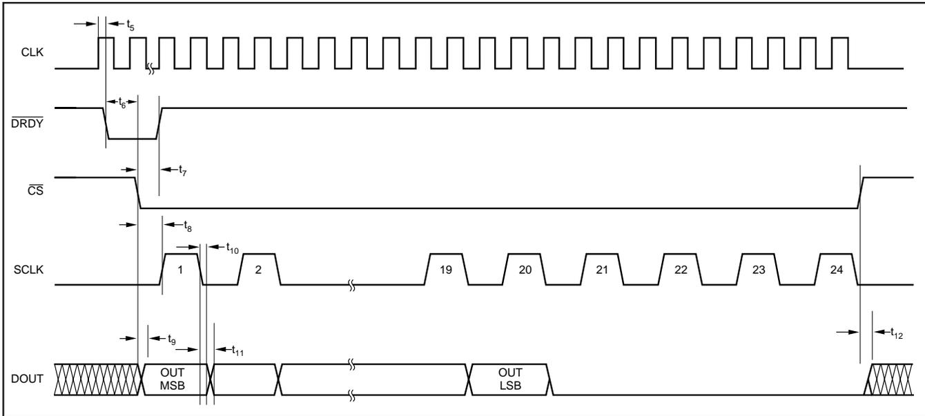
FIGURE 16. Method 1: Four-Wire Interface Using Noncontinuous SCLK.
