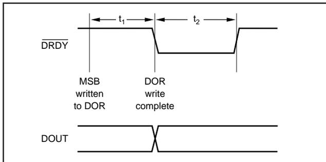
FIGURE 13.  $\overline{DRDY}$  Pulse ( $\overline{CS}$  tied LOW).
