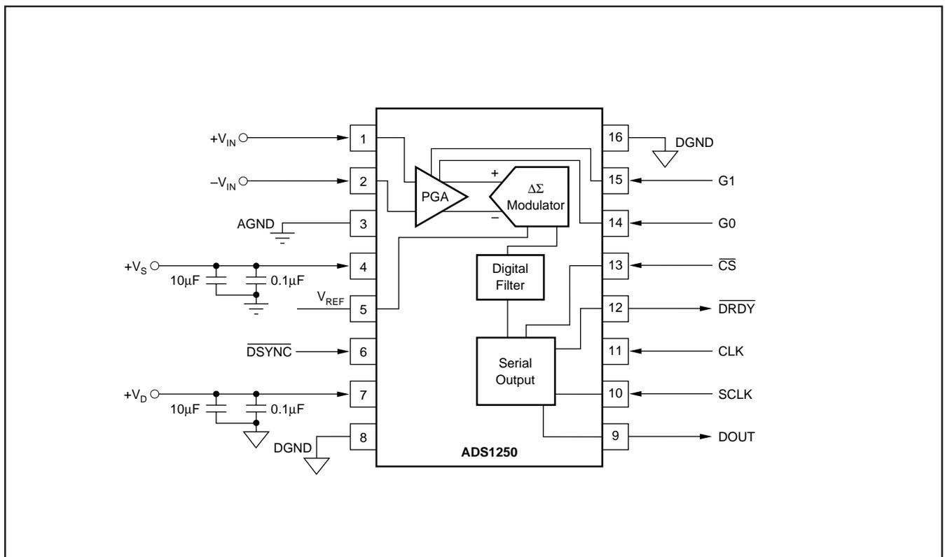
FIGURE 25. Connection Diagram.
