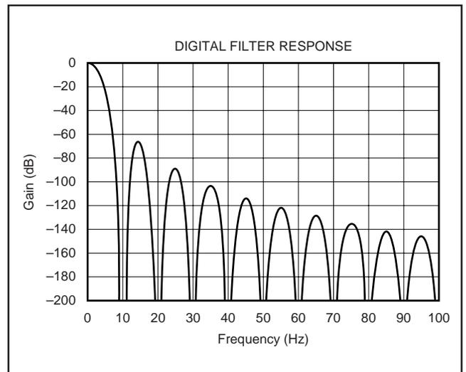
FIGURE 7. Digital Filter Response (10Hz).
