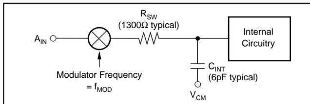
FIGURE 1. Analog-Input Structure.
