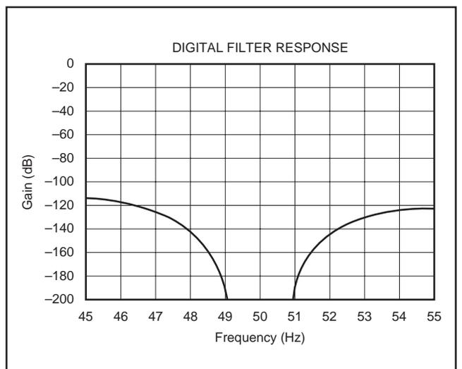
FIGURE 9. Expanded Digital Filter Response (50Hz with a 10Hz Data Output Rate).
