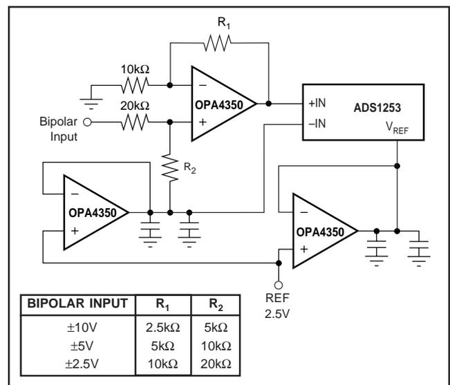
FIGURE 2. Level Shift Circuit for Bipolar Input Ranges.
