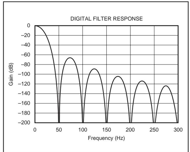
FIGURE 5. Digital Filter Response (50Hz).
