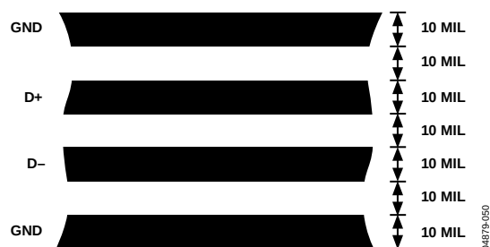
Figure 50. Arrangement of Signal Tracks
