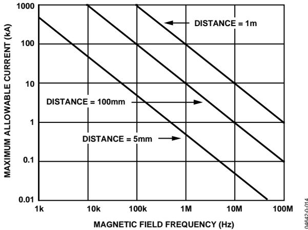
Figure 14. Maximum Allowable Current for Various Current-to-ADuM120x Spacings
