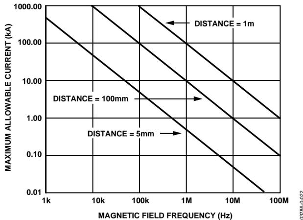
Figure 20. Maximum Allowable Current for Various Current-to-ADuM140x Spacings
