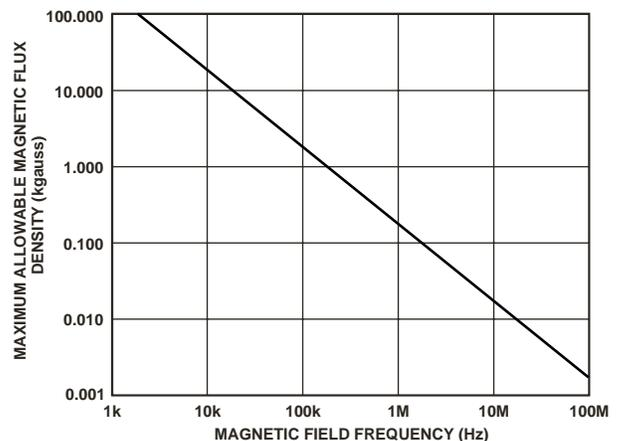
Figure 19. Maximum Allowable External Magnetic Flux Density
