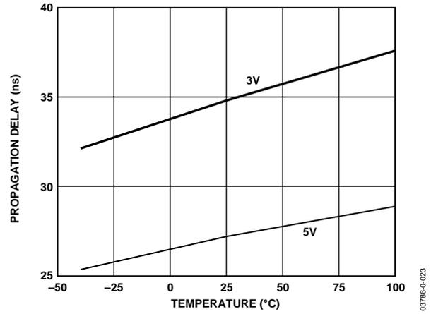
Figure 16. Propagation Delay vs. Temperature, C Grade
