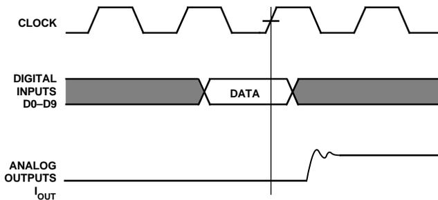
Figure 2. Video Data Input/Output
