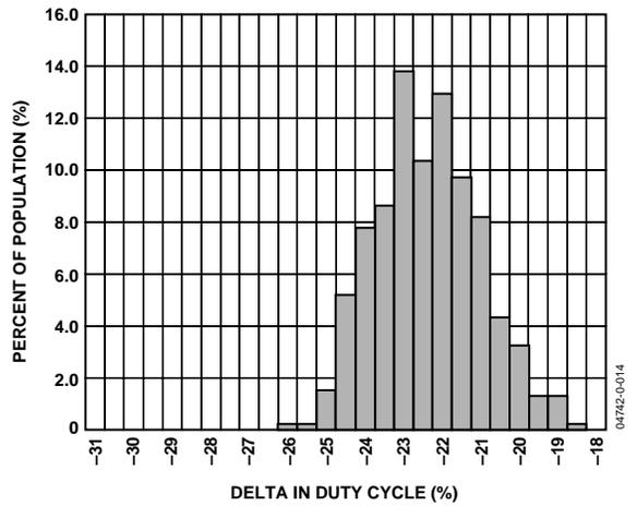
Figure 19. Y Axis Self Test Response at 25°C
