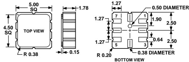
Figure 23. 8-Terminal Ceramic Leadless Chip Carrier [LCC]
