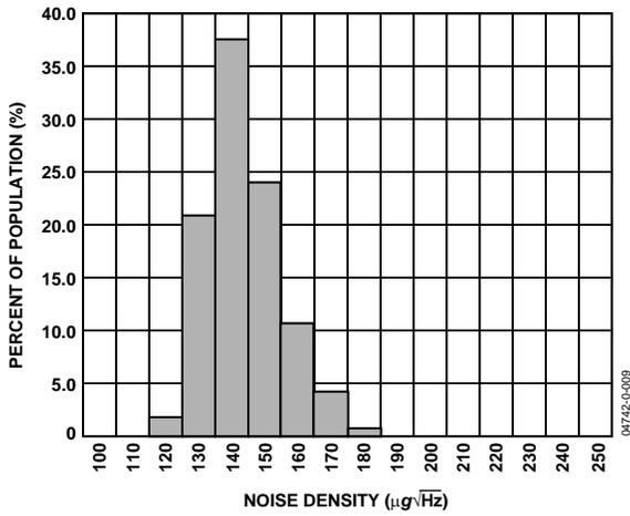
Figure 10. X Axis Noise Density at 25°C
