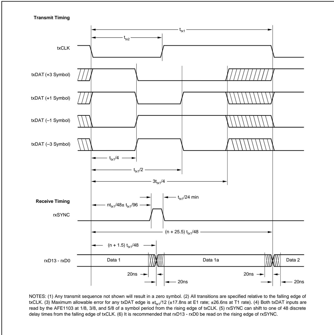
FIGURE 3. Timing Diagram.
