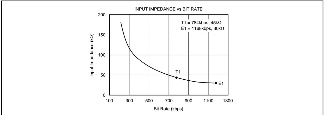
CURVE 3. Input Impedance of rxLINE and rxHYB.
