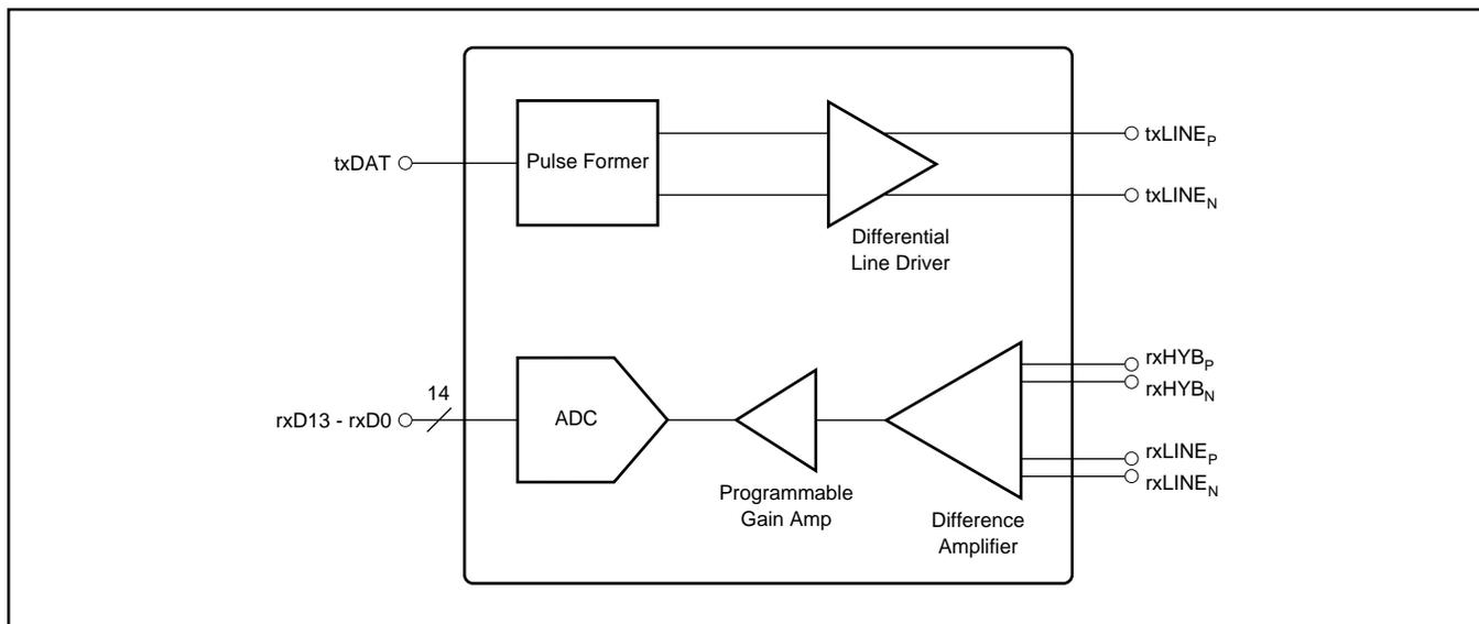
FIGURE 1. Functional Block Diagram of AFE1105.
