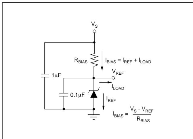
FIGURE 1. Typical Connections.
