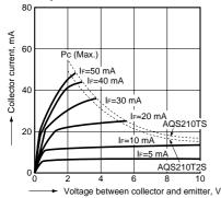
4-2. Collector current vs. voltage between collector and emitter characteristics (Ic-VcE) Measured portion: between terminals 6 and 7 (AQS210TS), (AQS210T2S)
