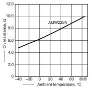
2.-(2) On resistance vs. ambient temperature characteristics
