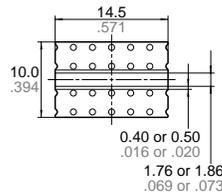
2) Material: Glass PTFE double-sided through hole PC board R-4737 (Matsushita Electric Works)
