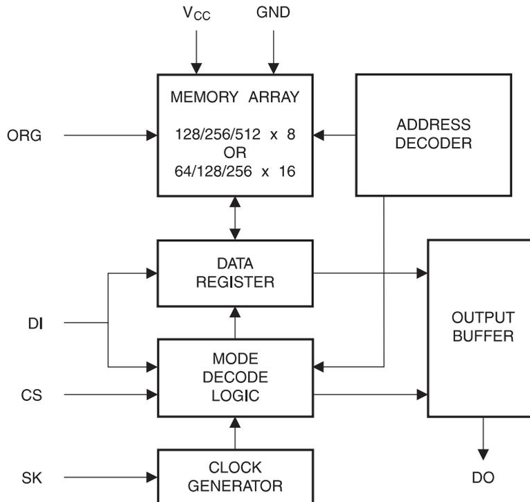
Note: 1. When the ORG pin is connected to  $V_{CC}$ , the x 16 organization is selected. When it is connected to ground, the x 8 organization is selected. If the ORG pin is left unconnected, then an internal pullup device (of approximately 1 M $\Omega$ ) will select the x 16 organization. This feature is not available on 1.8V devices.
