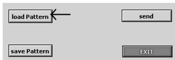
4. Select one of the .dat files (see [Figure 6-3 on page 13](#)). The ATA5283.dat protocol consists of a preamble followed by data which will be indicated by LED. In contrast, the ATA5282 requires, in addition, a header ID after the preamble before data are sent. These patterns are offered by ATA5282.dat file.
