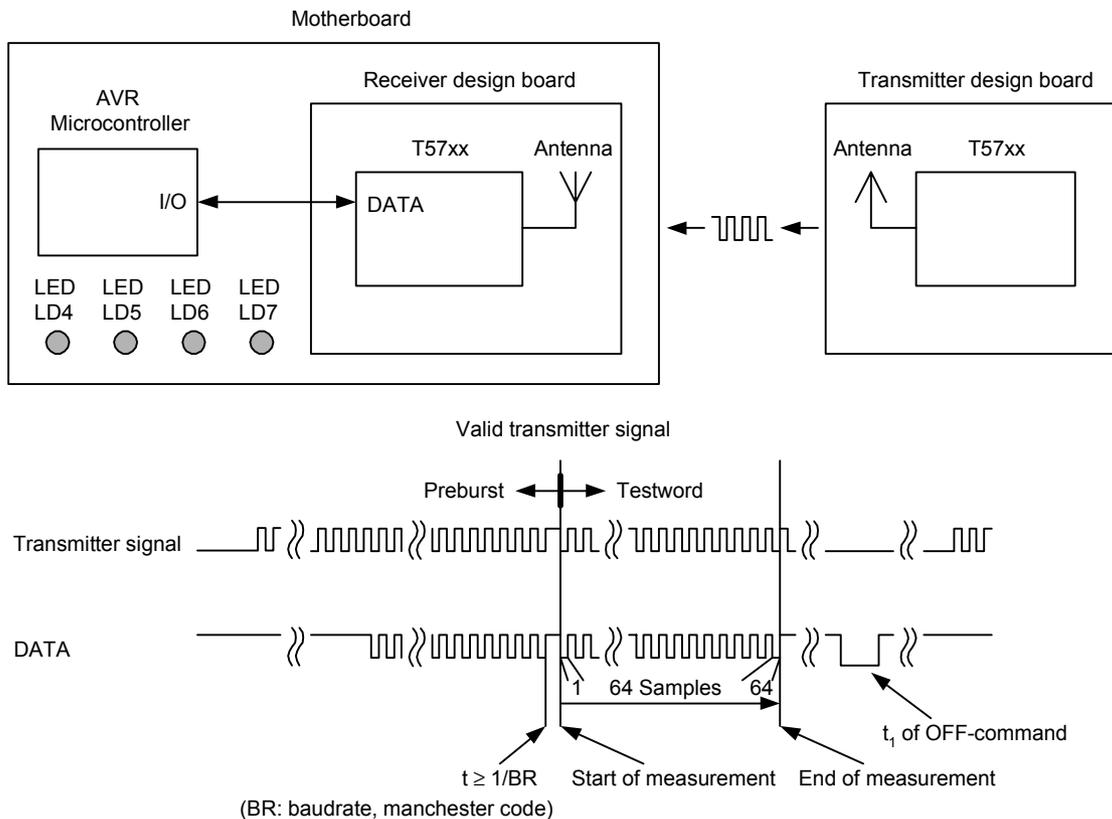
The AVR microcontroller continuously measures the time between two signal edges (= 1 sample). If the time  $t \geq 1/\text{baud rate}$ , the following 64 samples will be stored in the RAM of the microcontroller (start of measurement/end of measurement, see Figure 6 on page 7). Then, the RF receiver will be set back to polling mode by the microcontroller pulling pin DATA to '0' for a time  $t_1$ . The timing limits of  $1/\text{baud rate}$  are programmable in the RF Design Kit software.
