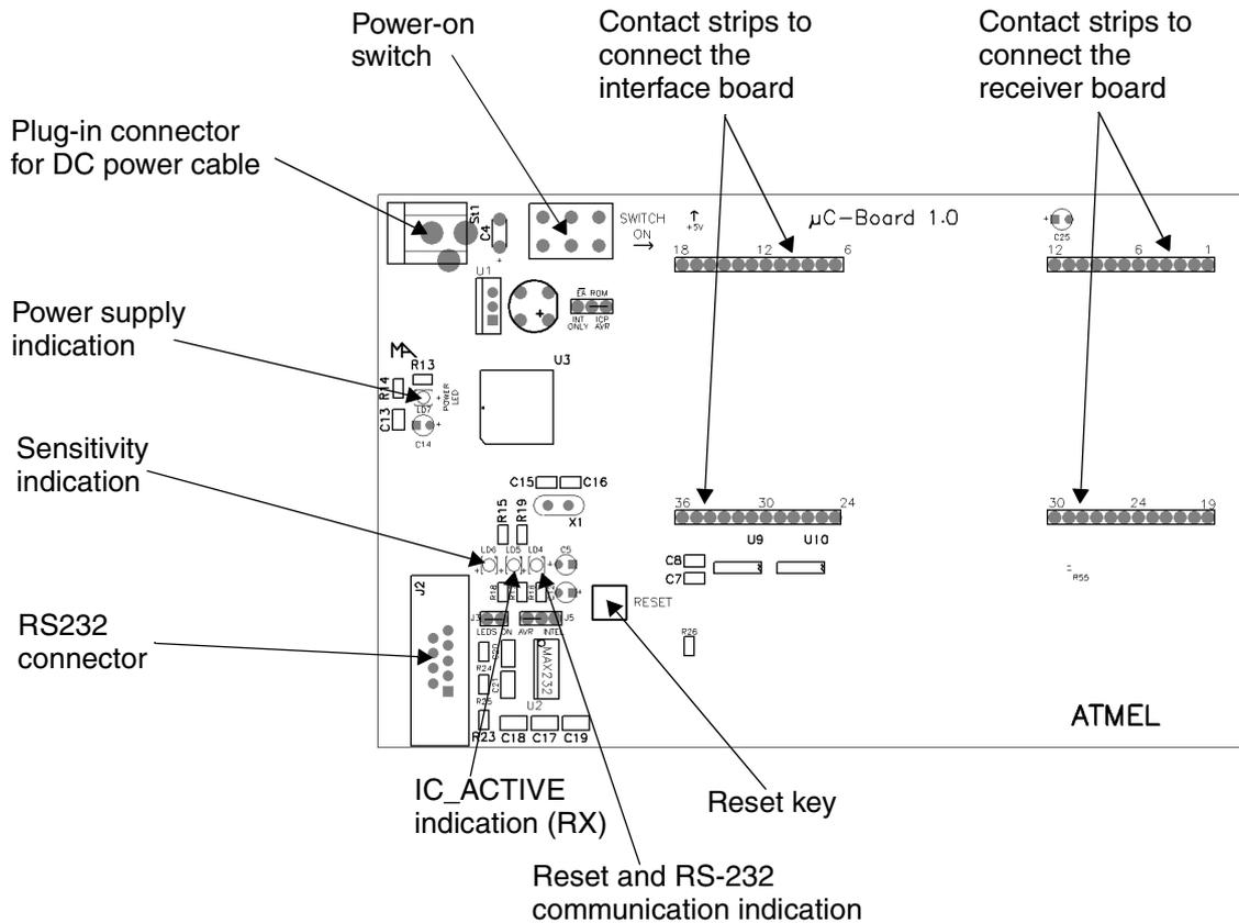
**Table 1.** Function of the LEDs on the Motherboard
