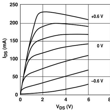
**Figure 1. Typical/Pulsed I-V Curves<sup>[6]</sup>.**
