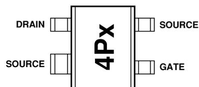
Note: Top View. Package marking provides orientation and identification.
