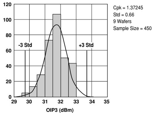
**Figure 2. OIP3 @ 2 GHz, 4 V, 60 mA.**
