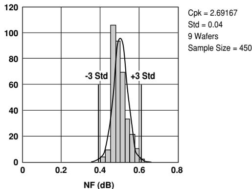
**Figure 3. NF @ 2 GHz, 4 V, 60 mA.**
