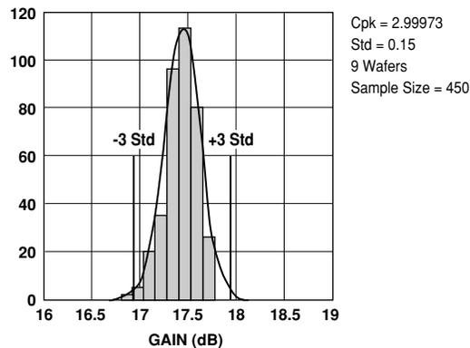
**Figure 4. Gain @ 2 GHz, 4 V, 60 mA.**
