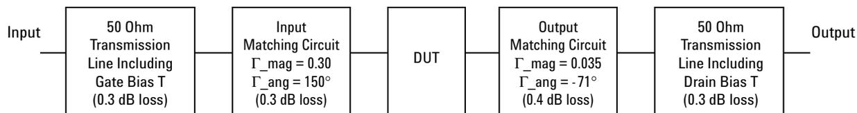
**Figure 5. Block diagram of 2 GHz production test board used for Noise Figure, Associated Gain, P1dB, and OIP3 measurements. This circuit represents a trade-off between an optimal noise match and associated impedance matching circuit losses. Circuit losses have been de-embedded from actual measurements.**
