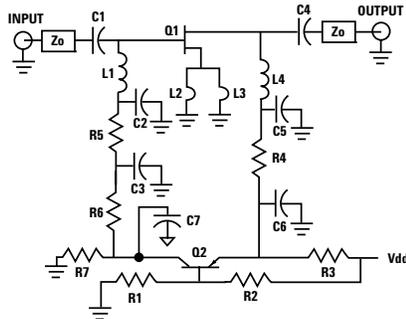
Figure 2. Typical ATF-54143 LNA with Active Biasing.
