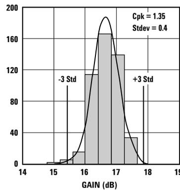
Figure 3. Gain @ 2 GHz, 3 V, 60 mA.
