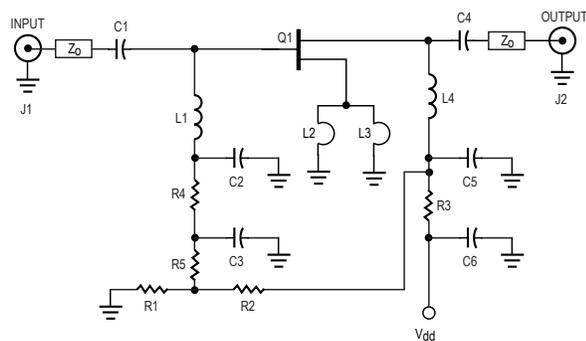
Figure 1. Typical ATF-54143 LNA with Passive Biasing.
