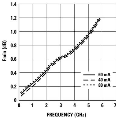
**Figure 18. Fmin<sup>[1]</sup> vs. Frequency and Ids at 3V.**
