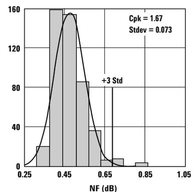
Figure 4. NF @ 2 GHz, 3 V, 60 mA.
