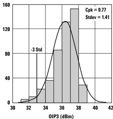
Figure 2. OIP3 @ 2 GHz, 3 V, 60 mA.
