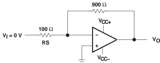
Figure 2. Noise-Test Circuit
