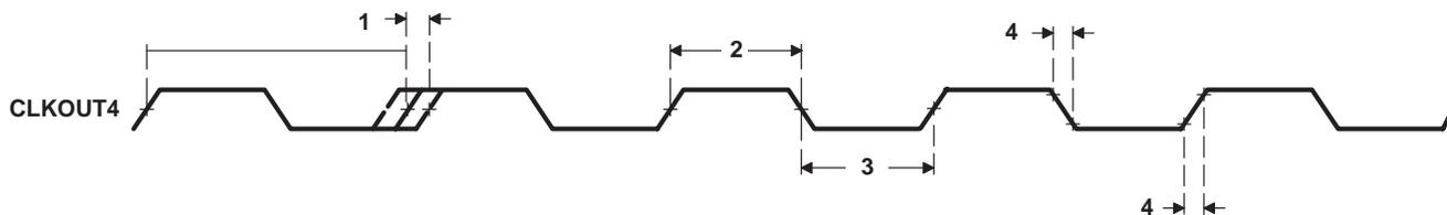
Figure 17. CLKOUT4 Timing
