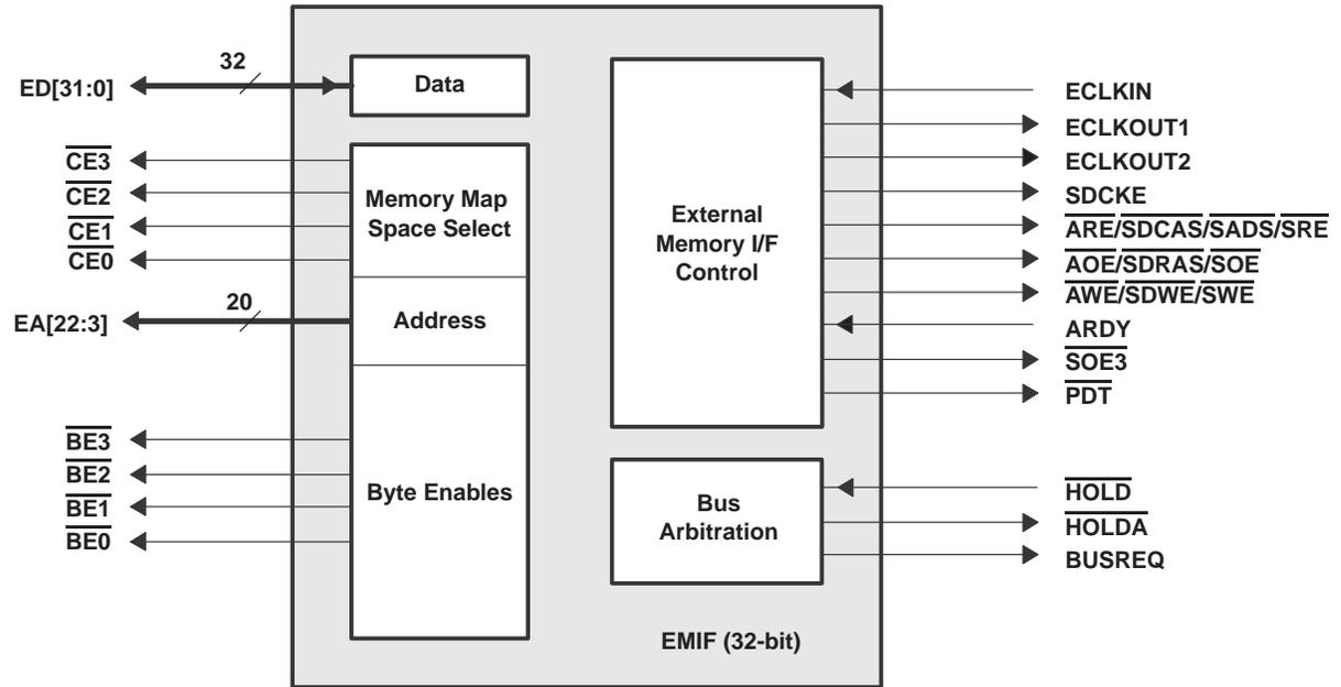
Figure 4. Peripheral Signals
