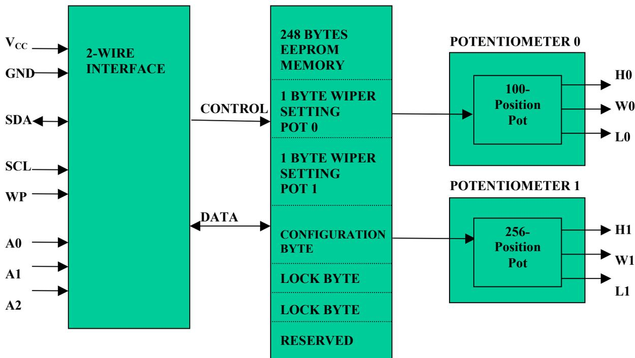
Up to eight DS1855s can be installed on a single 2-wire bus. Access to an individual device is achieved by using a device address that is determined by the logic levels of address pins A0 through A2. Additionally, the DS1855 will operate from 3V or 5V supplies. Three package options are available: 14-pin TSSOP, 16-ball STPBGA, and flip-chip package.
