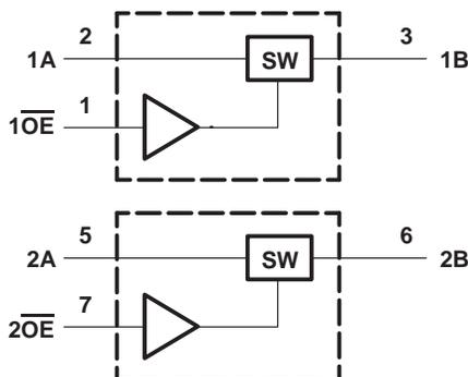
2.5-V/3.3-V LOW-VOLTAGE BUS SWITCH WITH 5-V TOLERANT LEVEL SHIFTER
