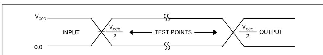
**NOTE:** AC test inputs are driven at  $V_{CCQ}$  for a logic “1” and 0.0V for a logic “0.” Input timing begins, and output timing ends, at  $V_{CCQ}/2$ . Input rise and fall times (10%–90%) <10 ns. Worst case speed conditions are when  $V_{CCQ} = V_{CCQMin}$ . 0580\_05
