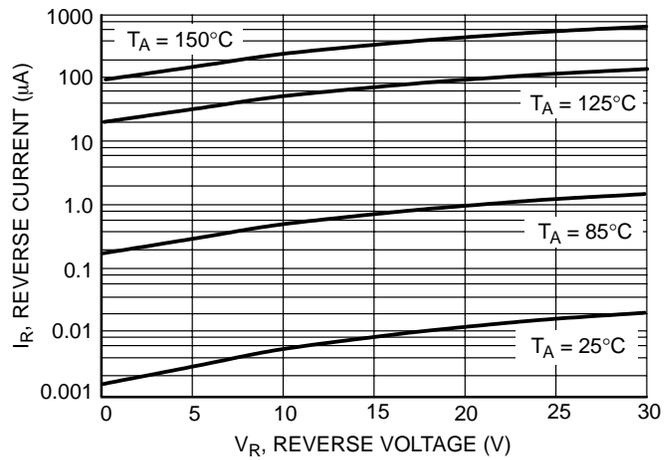
Figure 3. Leakage Current
