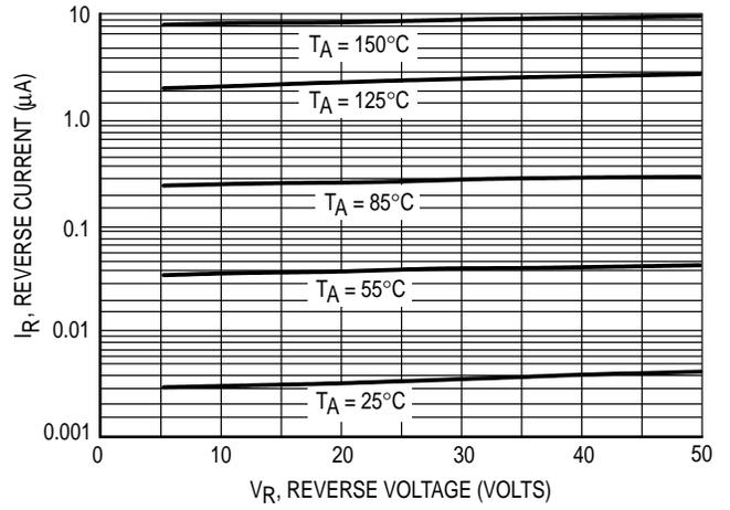
Figure 2. Leakage Current
