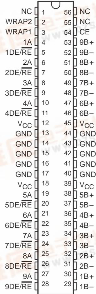
Pins 13 through 17 and 40 through 44 are connected together to the package lead frame and signal ground.
