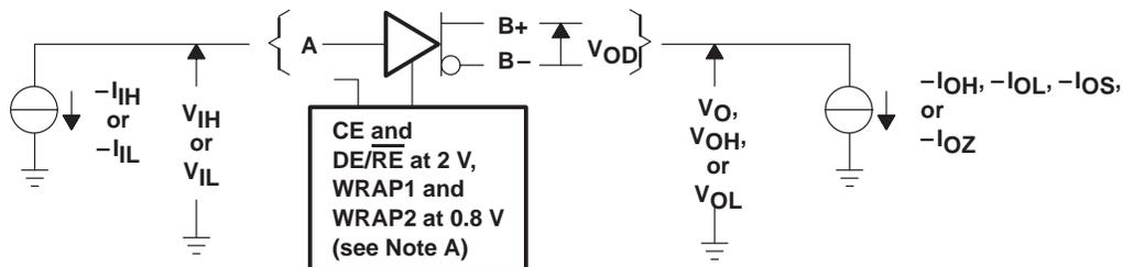
NOTE A: For the I<sub>OZ</sub> test, the CE input is at 0.8 V.
