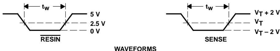
Figure 2. Input Pulse Definition
