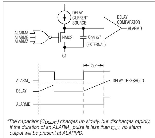
\*The capacitor ( $C_{DELAY}$ ) charges up slowly, but discharges rapidly. If the duration of an  $ALARM_{\_}$  pulse is less than  $t_{DLY}$ , no alarm output will be present at ALARMD.
