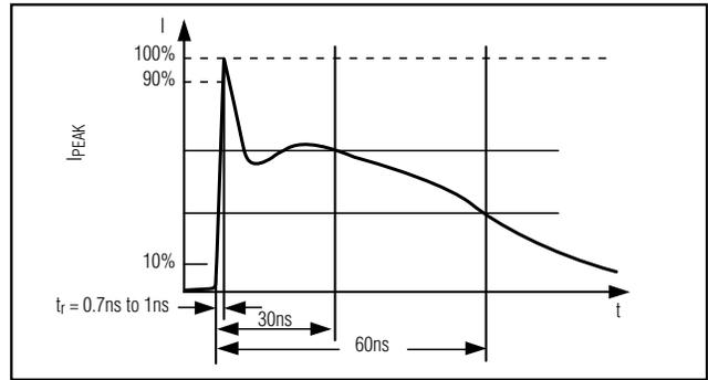
Figure 6b. IEC 1000-4-2 ESD Generator Current Waveform
