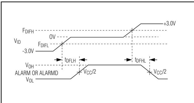
Figure 3. Fault-Detection Timing
