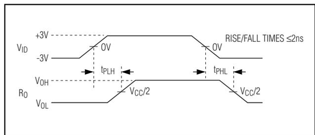
Figure 2. Propagation Delay
