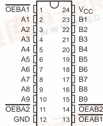
SN54BCT29863B ... FK PACKAGE (TOP VIEW)
