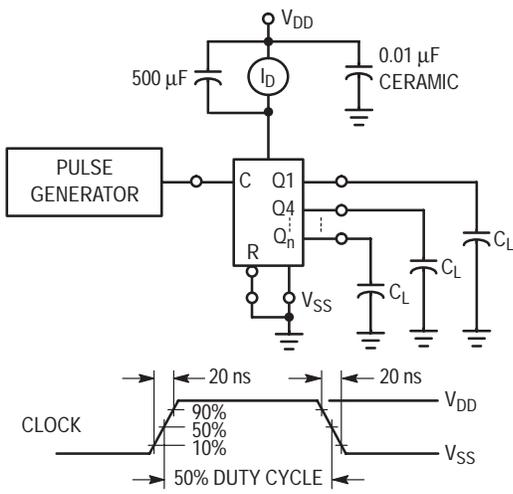
**Figure 1. Power Dissipation Test Circuit and Waveform**
