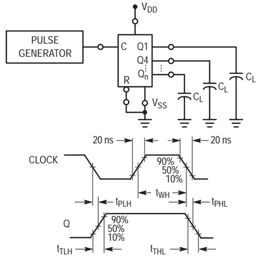
**Figure 2. Switching Time Test Circuit and Waveforms**
